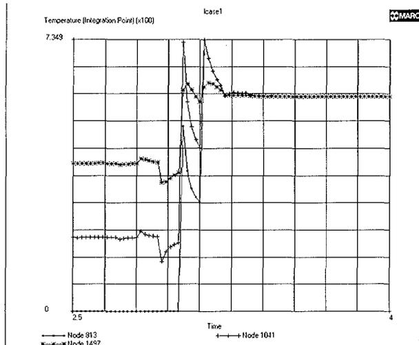
Fig.7. Dynamics of temperature variation on the top of the coating (node 813), in the interface (node 1041) and on the back side of substrate (node 1497)
