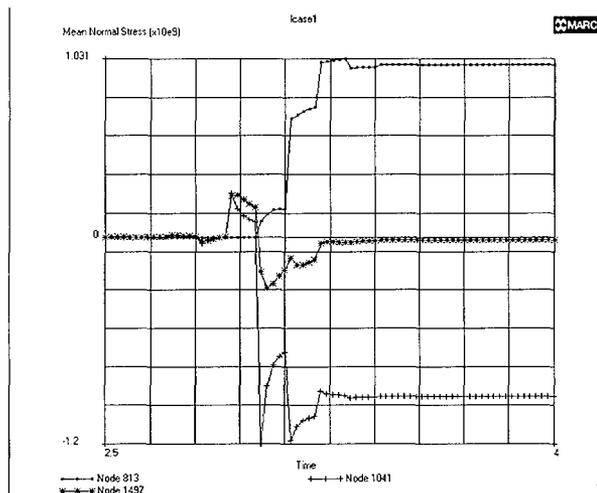
Fig.8. Normal stress dynamics in various points in the thickness of the system (without cracking)
