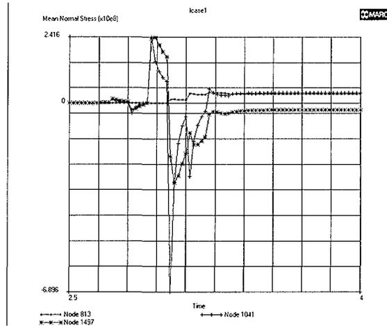
Fig.9. Normal stress dynamics in various points in system height (with cracking)
