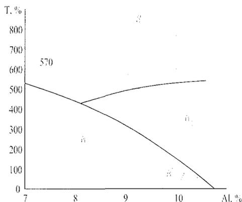
Fig. 1. Sequence of diffusionless transformations leading to formation of metastable phases in the sprayed structures of the Cu-Al system
