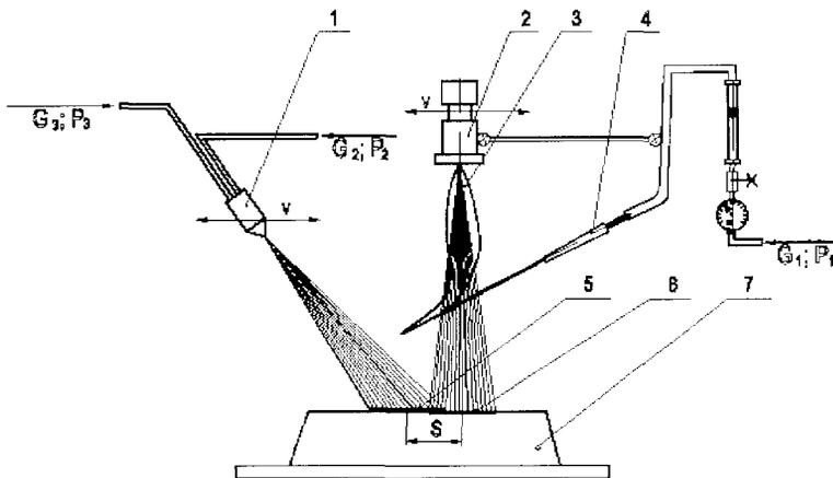
Fig. 2. Schematic of the cooling system: 1 - coolant sprayer; 2 - plasmatron; 3 - dusted plasma jet; 4 - slot nozzle of the blowing off system; 5 - cooling spot; 6 - spraying spot; 7 - model;  $v$ ,  $G_1$ ,  $G_2$ ,  $G_3$ ,  $P_1$ ,  $P_2$ ,  $P_3$  and  $S$  - process parameters of the cooling system
