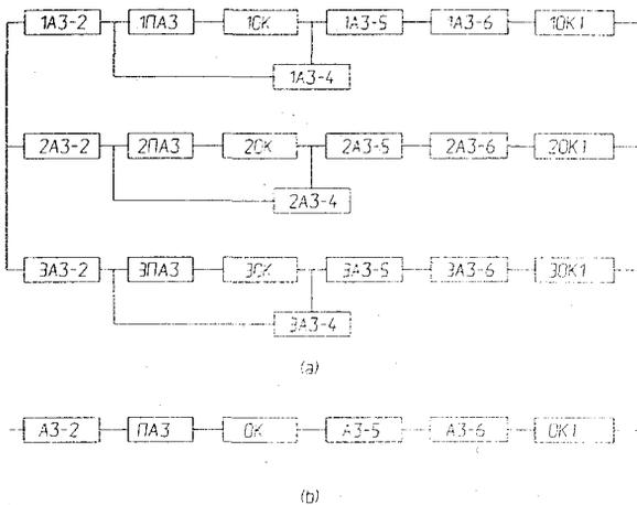
Fig.2. Reliability model of a safety injection system of units 3&4 of KNPP (a) and its pseudo-component "approximation" (b)
