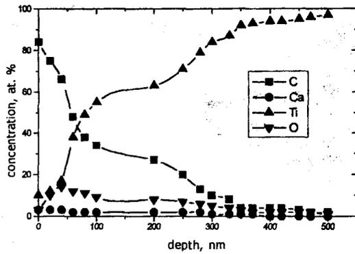
Fig. 6. Element distributions on a depth of the dental implant after irradiation (TEMP accelerator,  $E=300$  keV;  $\tau=50$  ns;  $n=5$  pulses;  $j=120-150$  A·cm<sup>-2</sup>).
