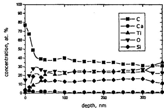
Fig.5. Element distributions on a depth of the dental implant after surface plastic straining (registration from the zone contained the conglomerate in Fig. 2).
