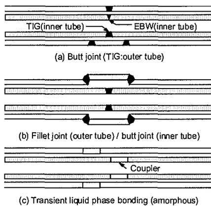
Figure 4 Tube-to-tube welding
