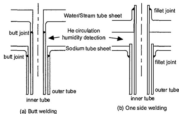
Figure 5 Tube-to-tube-sheet welding
