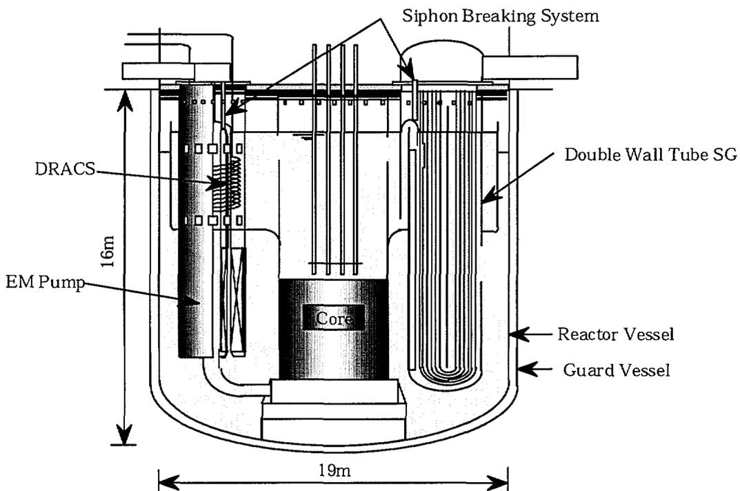
Figure 1 Schematic Diagram of ARES
