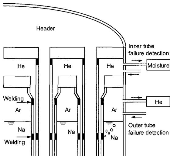
Figure 3 Schema of double-wall-tube structure
