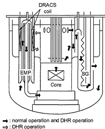
Figure 2 Coolant flow path
