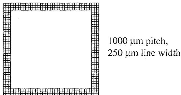
Figure 4 - View of the photo-lithographic fishbone grid deposit all around the screen. The external grid dimensions are about  $40 \times 40 \text{ mm}^2$ . The useful screen area for the laser spot reconstruction is the inner part of the grid.
