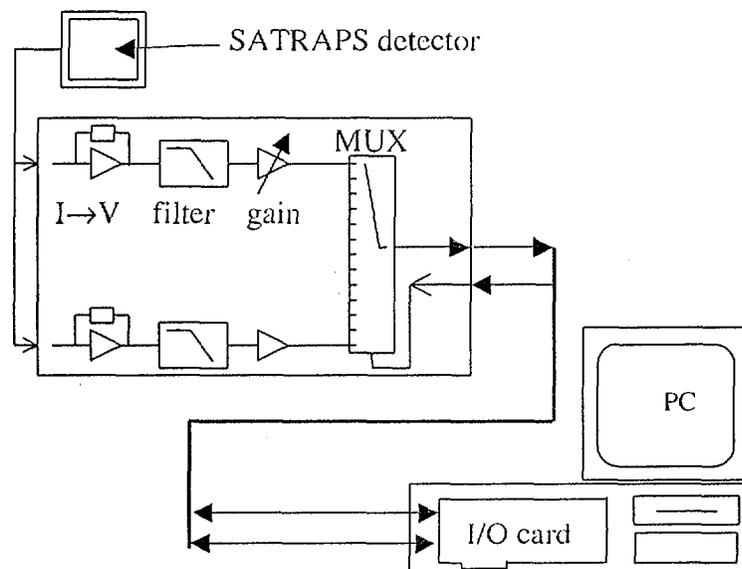
Figure 10 - Electronics readout chain of the photodiodes.
