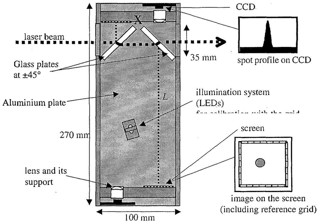
Figure 1 - Sketch of a STAMP showing the two arms. The three-point kinematic mount is located under the aluminium plate (sections 3 and 4). The role of the reference grid is explain in section 4.  $L$  is approximately equal to the distance between the glass plate and the screen of the long-arm (see text next page).
