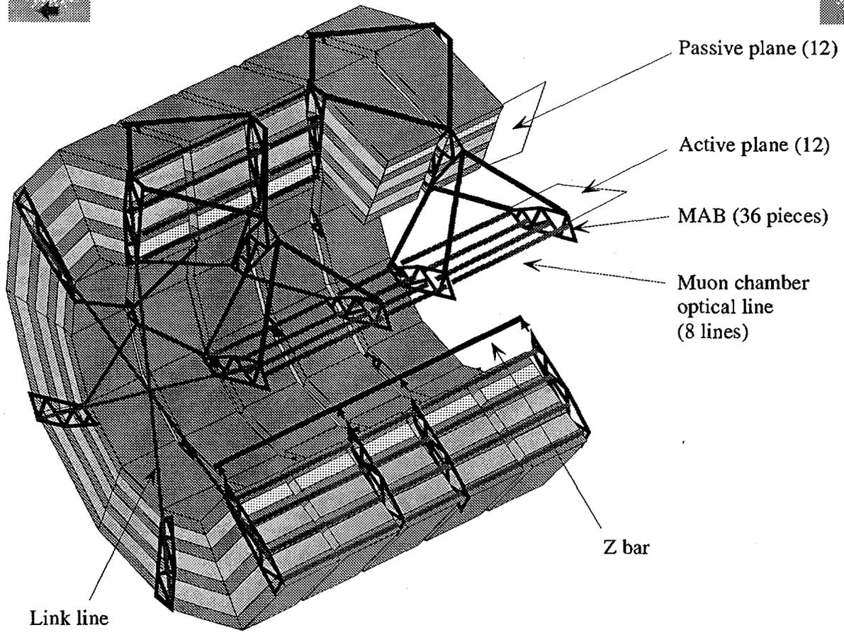
Figure 2 -A limited 3D view of the muon barrel spectrometer, the MAB structures, active planes and other local alignment elements are shown.
