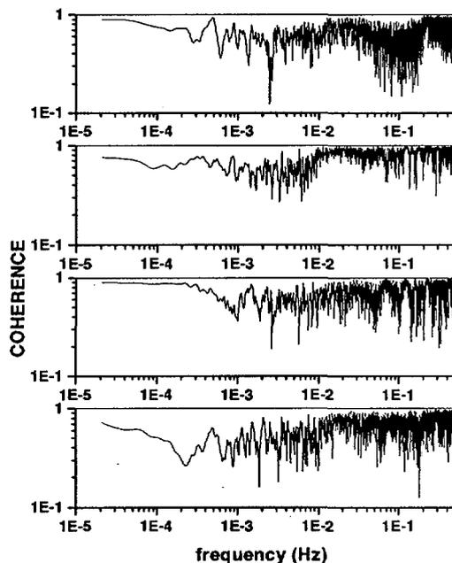
Figure 6: Coherence obtained in the quiet granite tunnel. Two sensors are set up 17 m apart from each other.
