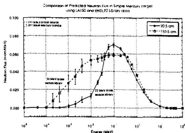
Fig.3. Neutron flux in 2-cm radius mercury target.
