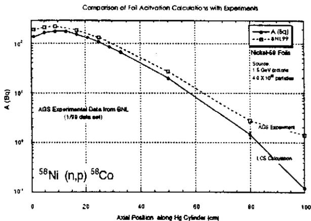
Fig. 14. Comparison of predicted and measured activity in a nickel foil due to (n,p) reactions.
