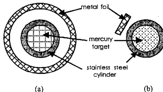
Fig. 12 Schematic transverse cross-sections of (a) annular and (b) discrete AGS foil models.
