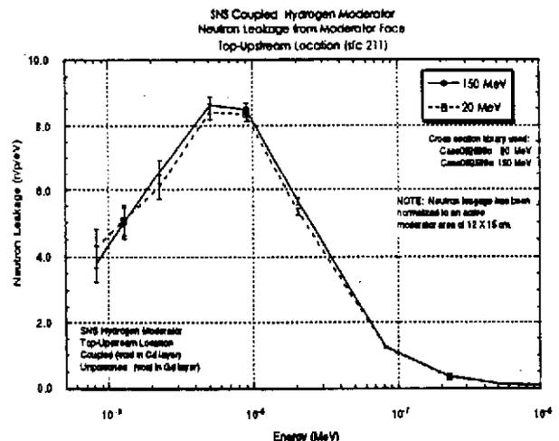
Fig. 10. Comparison of predicted neutron leakage from a coupled hydrogen moderator.
