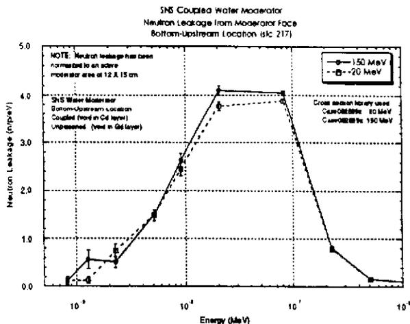
Fig. 11. Comparison of predicted neutron leakage from a coupled water moderator.
