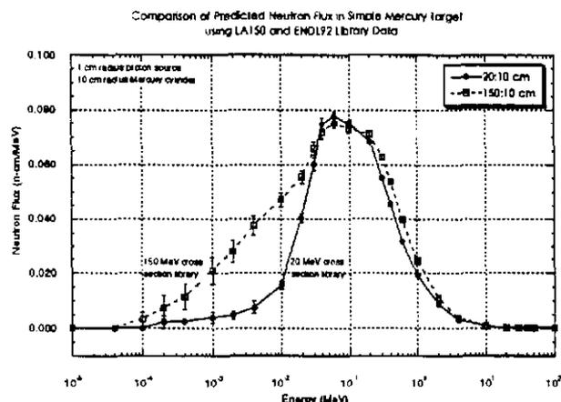
Fig.5. Neutron flux in 10-cm radius mercury target.
