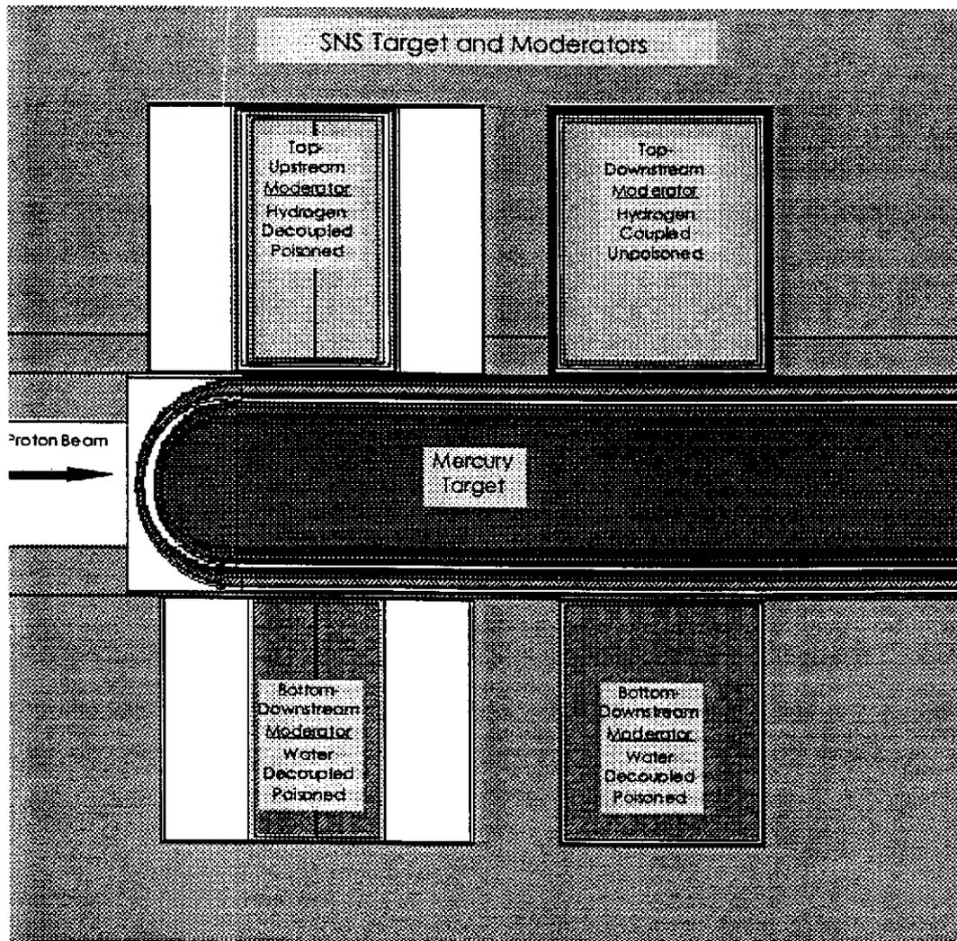
Fig. 7. Cross-section of MCNP geometrical model of SNS target and moderator region.
