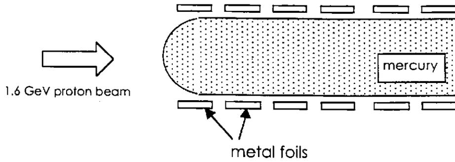
Fig. 13. Schematic axial cross-section of the geometric model used in LAHET, HMCNP and MCNPX to simulate foil activation experiments in the AGS experiments.
