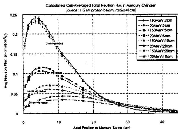
Fig. 1. Axial profile of neutron flux in simple cylindrical mercury targets of various diameters.
