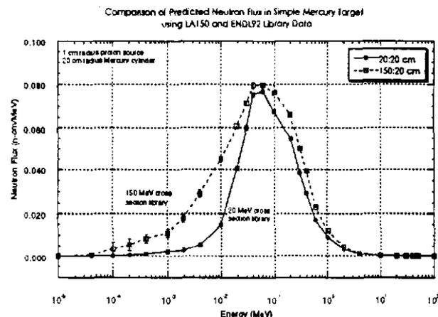
Fig.6. Neutron flux in 20-cm radius mercury target.
