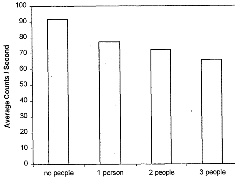
Figure 4.4. Changes in Observed Count Rate when Various Numbers of People are Located Between the Neutron Sources in a Storage Vault and the Detector
