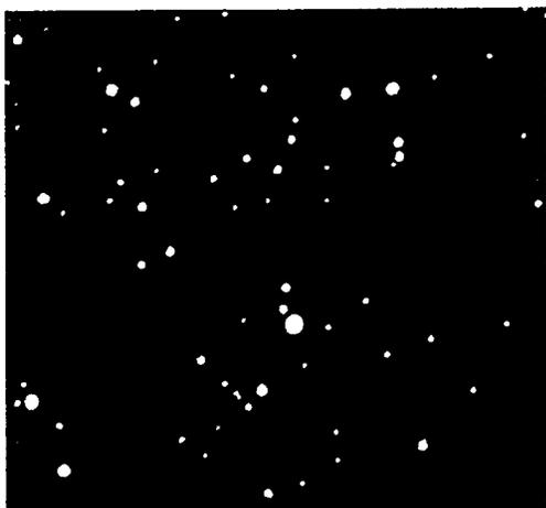
Fig. 6a. SEM photomicrograph showing particulates formed with pulse width of 27ns.
