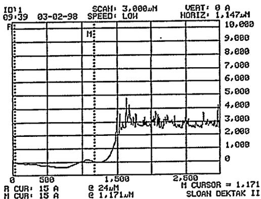
Fig. 5a. Profilometer traces of film thickness on silicon in oxygen atmosphere.
