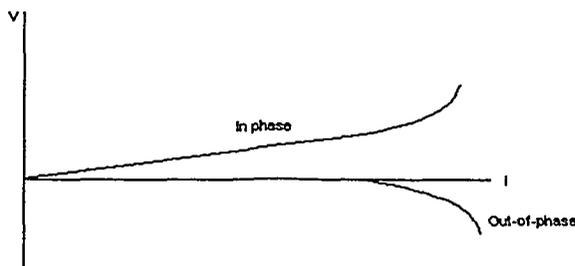
Fig. 2. Mutual inductance signal plotted against drive current.
