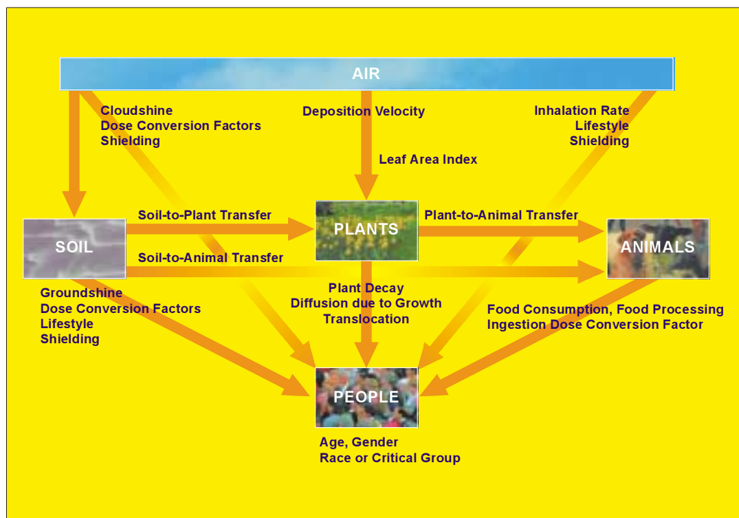
Figure 1: RadCon Exposure Pathways and some required data.
