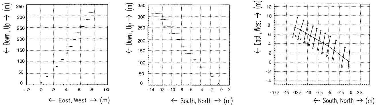
Figure 3: The left two plots represent a side view of the line during 17 days. It reveals an extremely stable behavior: the detector is almost straight and the horizontal relative displacement of each module is less than 3 m. The right plot is a top view of the prototype. The top spacer lays  $\sim 14$  m away from the vertical axis passing through the left of the demonstrator. The arrows display the measured heading of the spacers: the line does not seem to be twisted.
