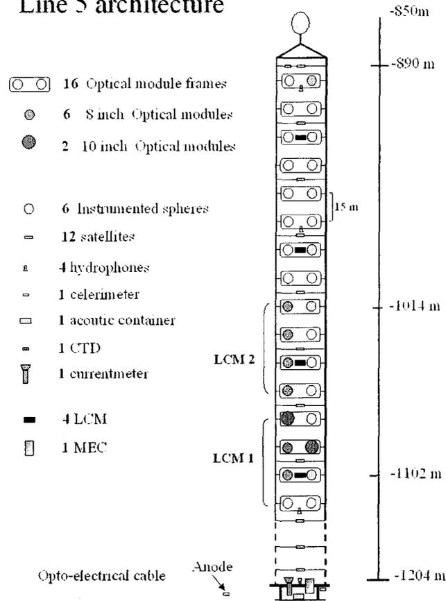
Figure 2: Demonstrator architecture
