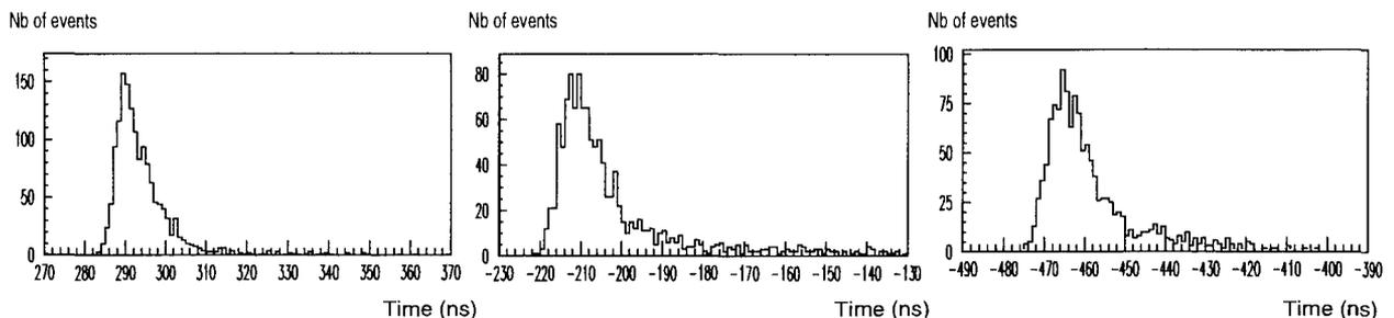
Figure 4: Histogram distribution of PMT time response illuminated by a LED with own pulsing jitter of 7.3 ns. From left to right the three histograms correspond to the three bottom PMT of the line. The asymmetry of the distribution is mainly due to diffusion process.
