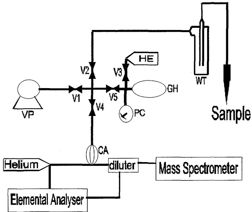
Fig. 1. Schematic representation of extraction equipment (WT – water trap [–90°C]; GH-gas reservoir[250ml]; VP – vac. pump; CA – capillary; V1..5 – valves; HE – helium; PC – pressure gauge.
