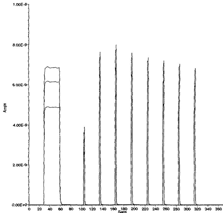
Fig. 2. Plot of a  $^{13}\text{C}/^{12}\text{C}$  run of carbon dioxide extracted from mineral water. The first peak is generated by the reference gas, the subsequent spikes are separate samples gas injections from the gas reservoir (see text).
