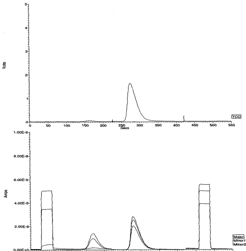
*Fig. 3. Run of atropin standard (upper part: TCD signal; lower part: mass spectrometric record of the gases exhausting from the EA., Nitrogen is eluting first, followed by the carbon dioxide) The chromatogram is bracketed by gas injections of  $\text{N}_2$  and  $\text{CO}_2$  reference gas respectively. Switching of the high voltage and hence the mass position occurs at 225 seconds.*
