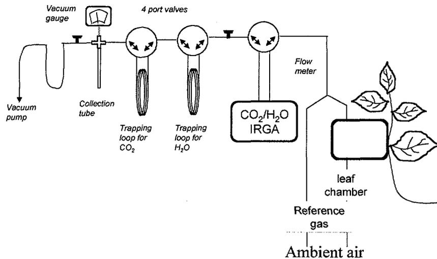
Fig. 2. On-line sampling system for the field sampling of gases exchanged between leaves and atmosphere. An attached leaf is enclosed in a leaf cuvette and an air stream is sampled before and after passing above the leaf. Water vapor and CO<sub>2</sub> concentrations are measured by an infra-red-gas analyzer, water is trapped at -8°C and CO<sub>2</sub> at -170°C. Samples are cryogenically transferred to a collection tube for the mass spectrometric analysis.
