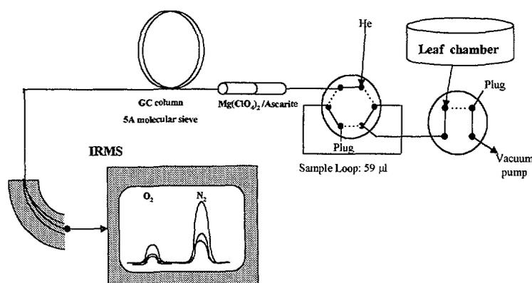
Fig. 5. On line sampling and analysis system for O<sub>2</sub> isotopic composition during respiration.
