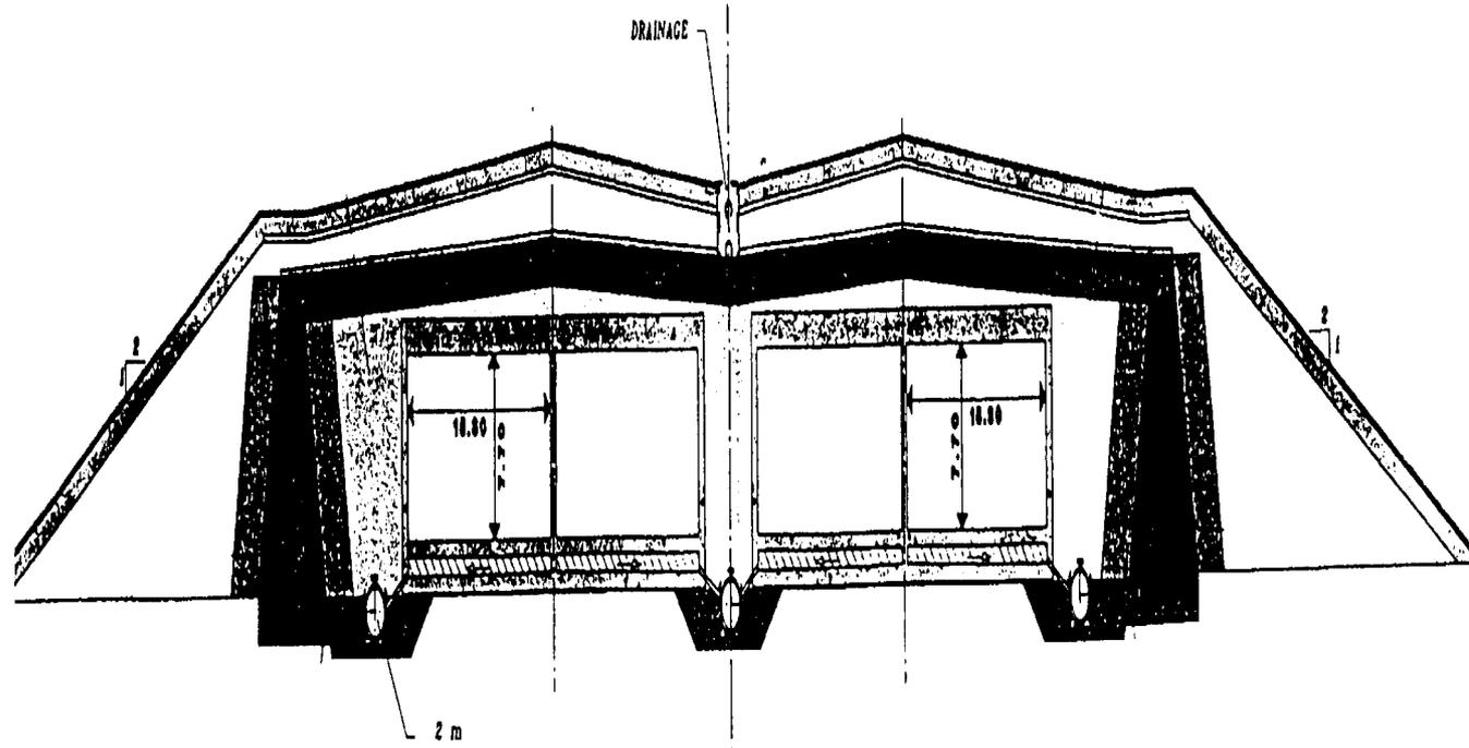
FIG. A.6. Basic design of new repository for conditioned radioactive waste.
