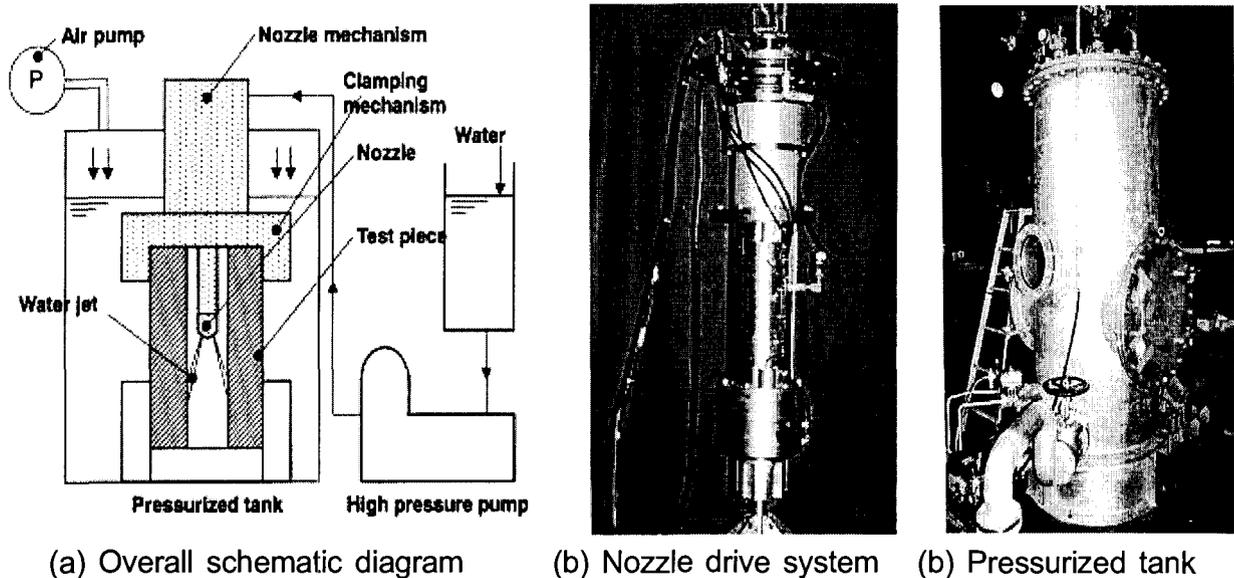
Figure 2. WJP test apparatus
