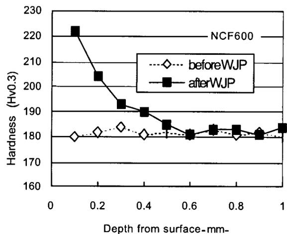
(b) Measured hardness of section near surface after WJP
