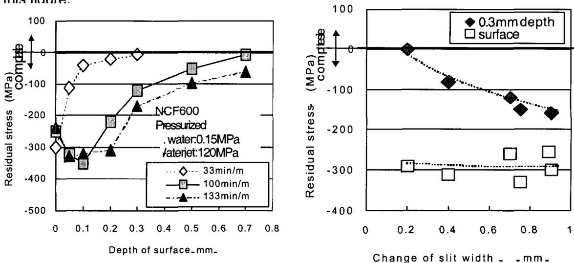
(a) Peening time vs. residual stress      (b) Relation between slit width and residual stress
