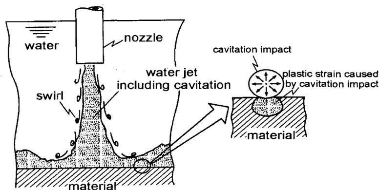
Figure 1. Model diagram of WJP Using Cavitation
