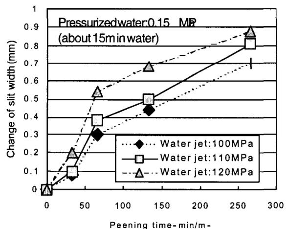
Figure 5. Change in slit width of pipe due to WJP
