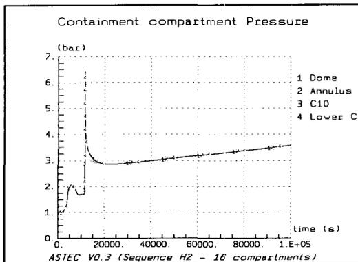
Figure 7: containment pressure – without spray
