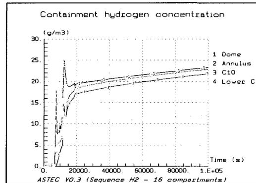
Figure 16: hydrogen concentration – with spray
