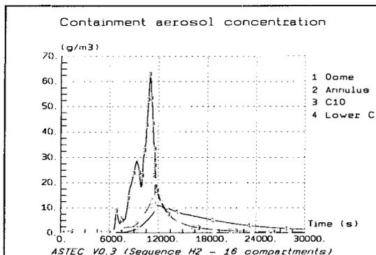
Figure 17: aerosol concentration– without spray
