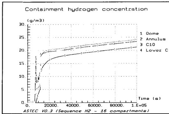
Figure 15: hydrogen concentration – without spray
