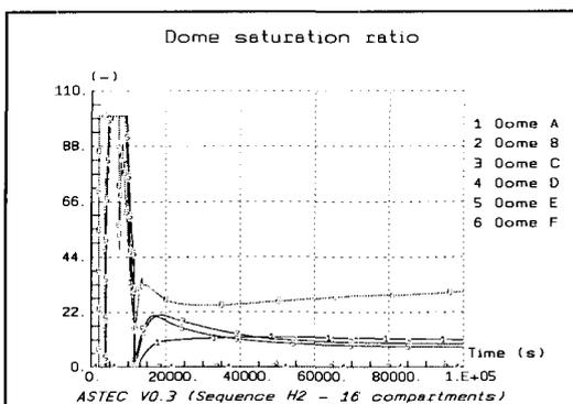
Figure 9: saturation ratios – without spray
