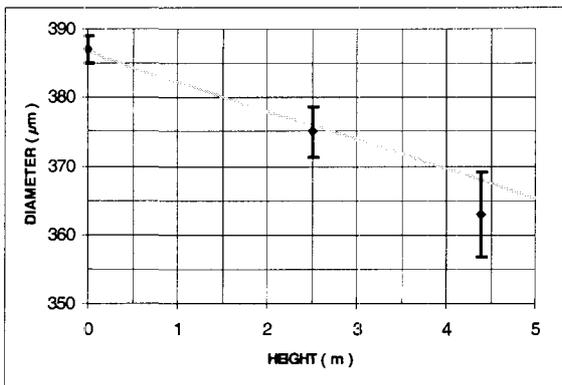
Figure 2 : droplet size evolution for a gas at 1 bar,  $47^\circ\text{C}$  and RH 12 %.
