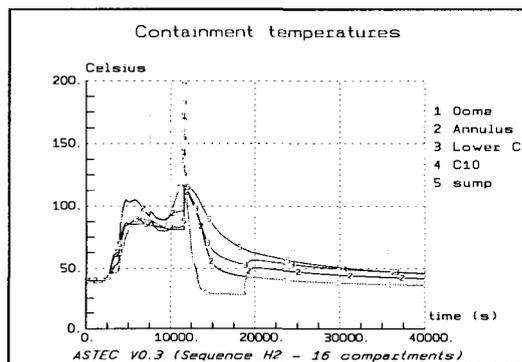
Figure 12: temperatures – with spray
