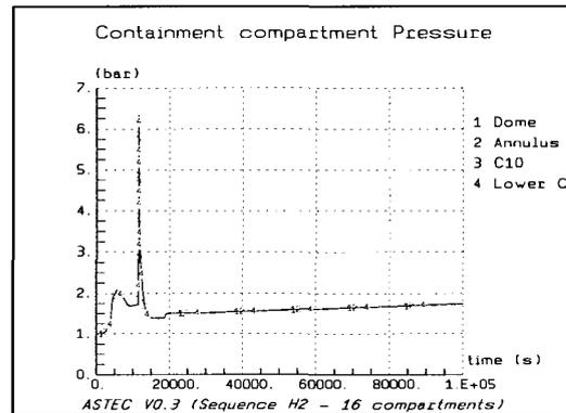
Figure 8: containment pressure – with spray
