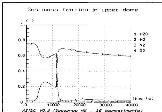
Figure 14: steam fraction – with spray
