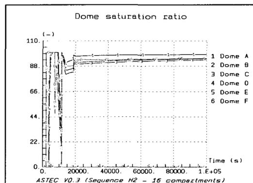
Figure 10: saturation ratios – with spray
