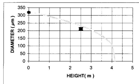
Figure 5 : droplet size evolution for a gas at 3.2 bar,  $135^\circ\text{C}$  and RH 2.3 %
