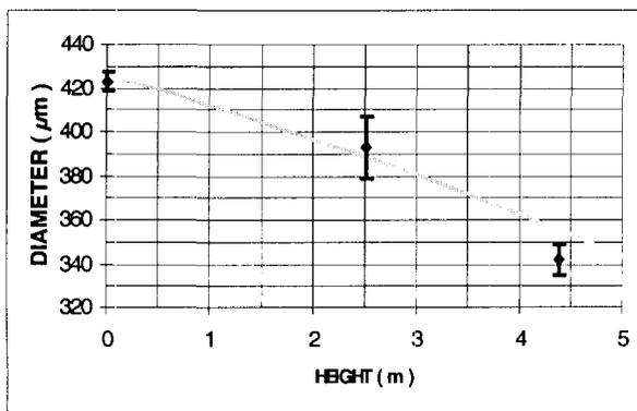
Figure 3 : droplet size evolution for a gas at 1 bar,  $146.6^\circ\text{C}$  and RH  $< 1\%$
