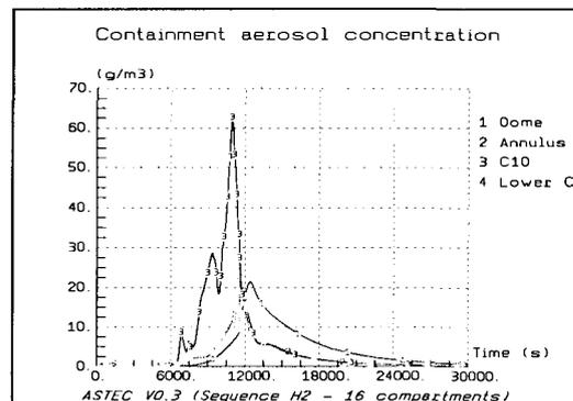
Figure 18: aerosol concentration– with spray
