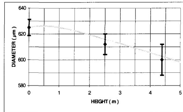
Figure 4 : droplet size evolution for a gas at 2.4 bar,  $99^\circ\text{C}$  and RH 6.3 %
