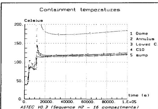
Figure 11: temperatures – without spray
