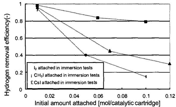
Fig. 4 Percentage of Drop in Hydrogen Removal Efficiency on Account of Reaction Inhibitors
