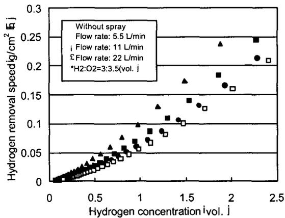
Fig.7 Containment Vessel Spray Performance Retention Tests
