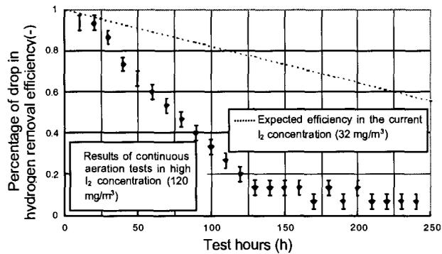
Fig. 5 Percentage of Drop in Hydrogen Removal Efficiency
