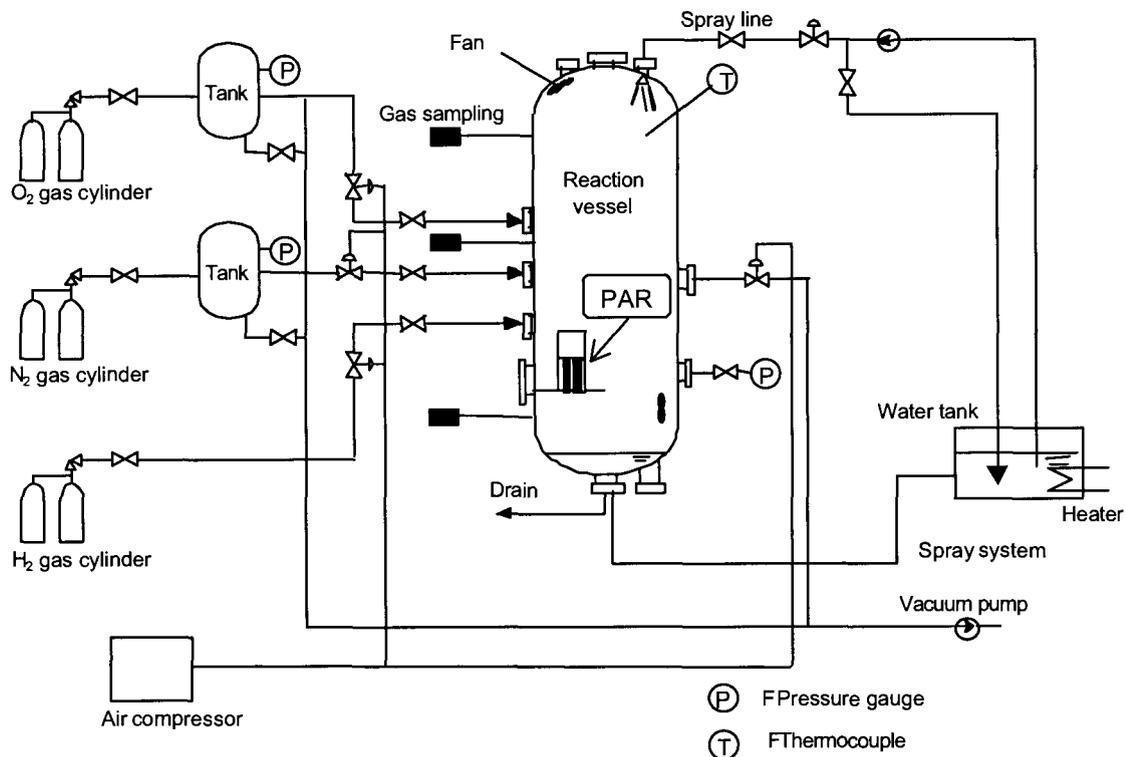
Fig. 6 A Schematic Diagram of the In-the-Vessel Spray Testing System
