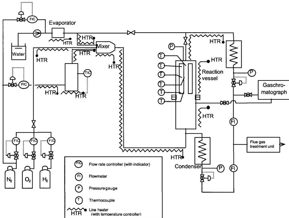
Fig. 3 A Schematic Diagram of the Single Catalyst Element Testing System
