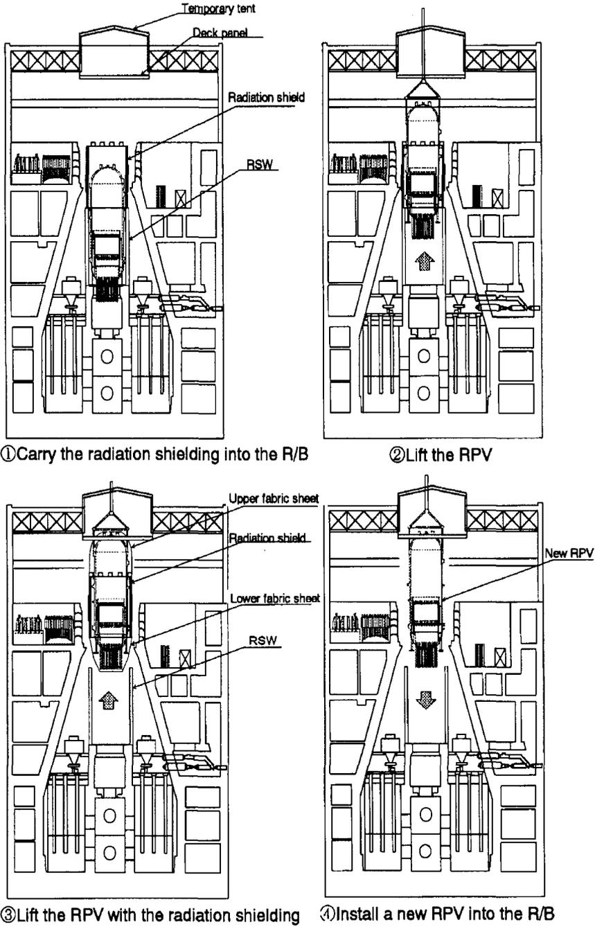
Fig.2 The method of lifting the RPV for 1100MWe class plant
