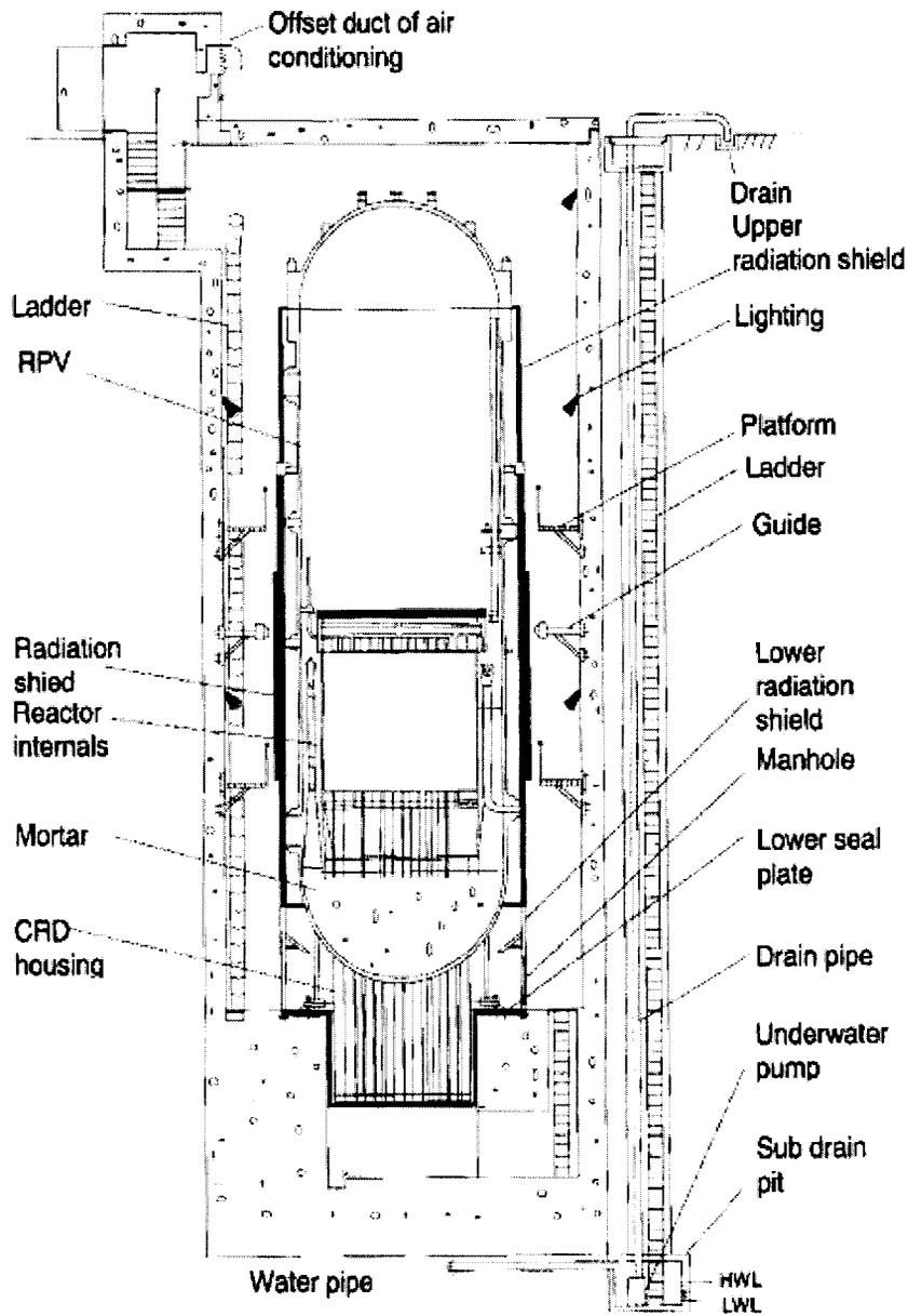
Fig.4 RPV storage pit (underground type)
