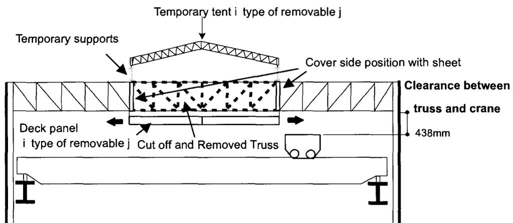
Fig.3 The method of making an opening in the top of R/B
