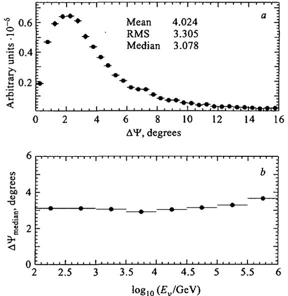
Fig. 5. Error in the space angle for simulated signal events with energy spectra proportional to  $E_{\nu}^{-2}$ : (a) distribution of error averaged over declination; (b) space angle error as a function of neutrino energy
