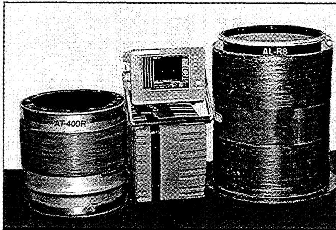
*FIG. 1. EM-Coil System used with AT400R and ALR-8 Storage Containers*
