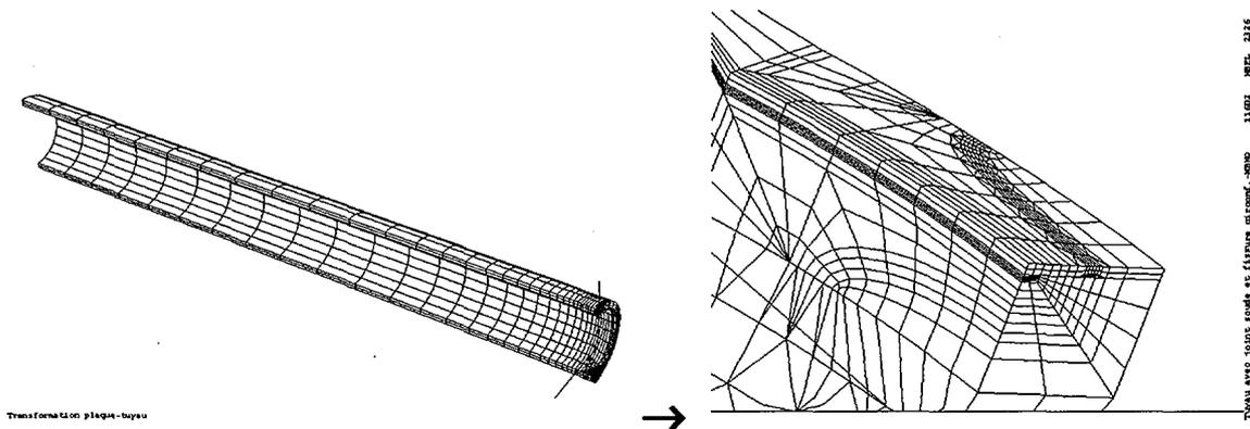
*FIGURE 7. Pipe mesh with zoom of the crack region*
