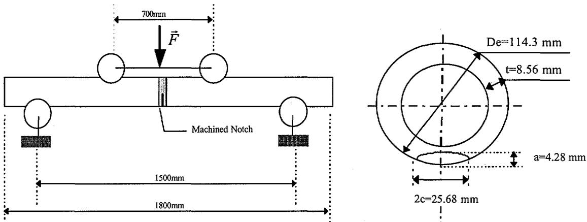
FIGURE 2. Notch location and shape
