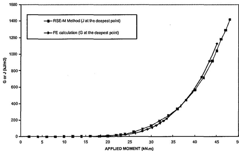
FIGURE 10. Comparison between finite element G and J obtained by RSE-M method
