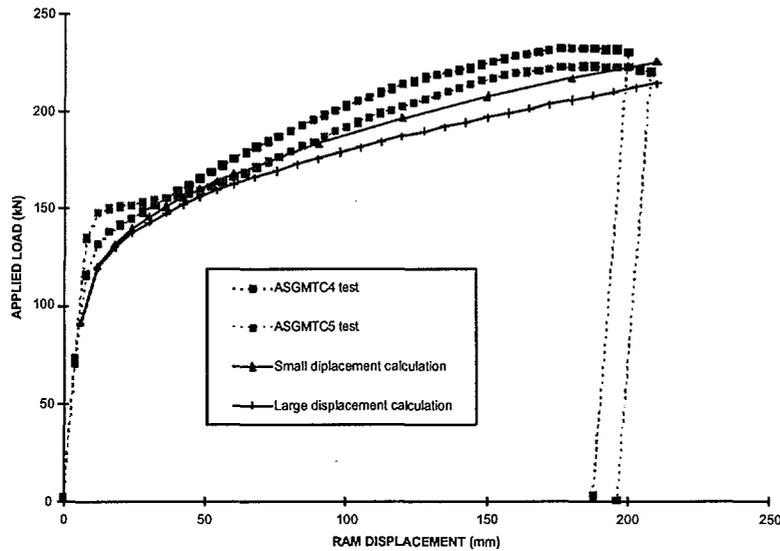
FIGURE 8. Applied load versus ram displacement (test and computation curves)
