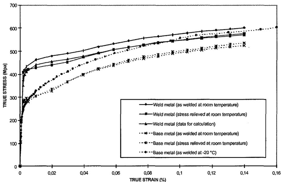
FIGURE 3. True stress - true strain curves for base and weld metal
