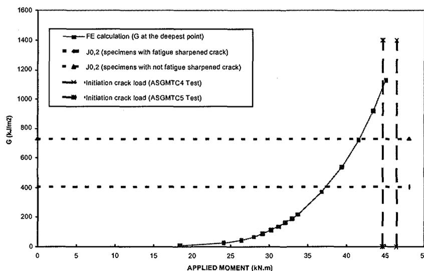
FIGURE 9. Crack initiation prediction with FE energy release rate
