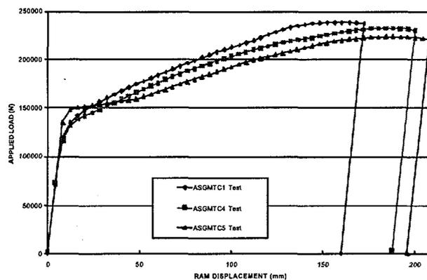
FIGURE 4. Applied load versus ram displacement (test curves)
