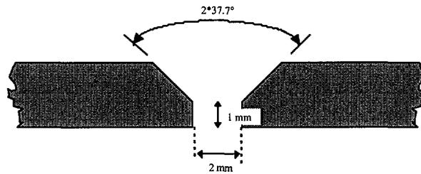
FIGURE 1. Specified dimensions of the V weld joint
