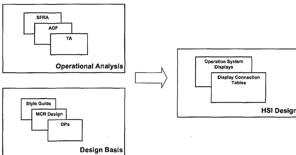
Figure 3: HSI Design Process
