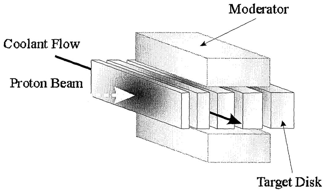
Fig.1 Schematic of the solid target
