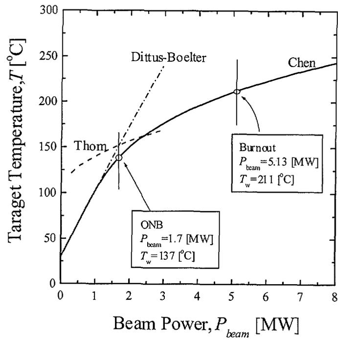
Fig.8 Temperature variation of solid target with beam power
