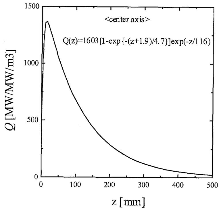
Fig.7 Heat generation density per beam power along the center axis of the target
