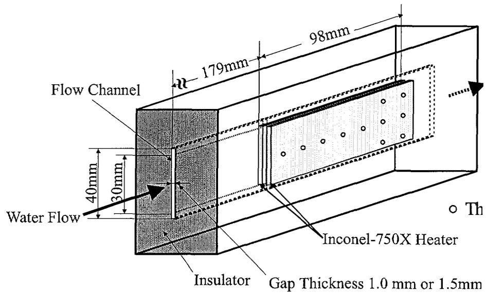
Fig.2 Cross sectional view of the test section
