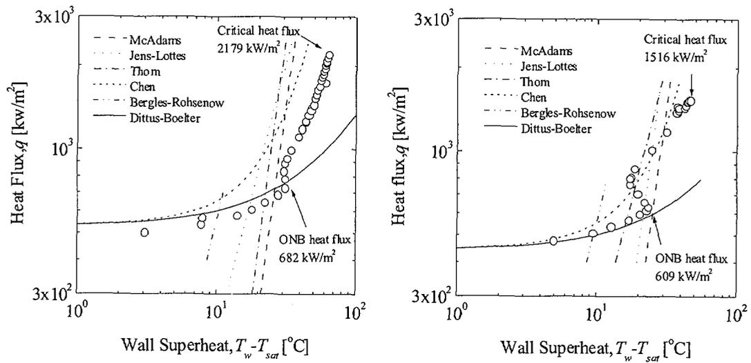
Fig.4 Typical result of boiling curve
