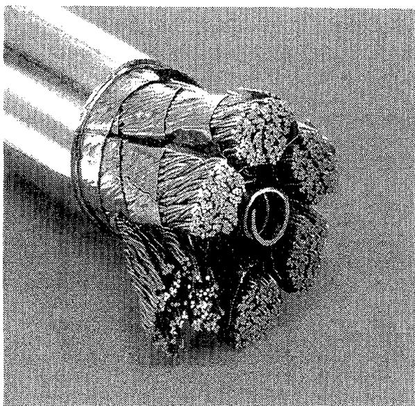
Fig. 1: TFMC conductor: 720 Nb<sub>3</sub>Sn and 360 Cu strands cabled around a centre spiral and inserted in a 316LN jacket
