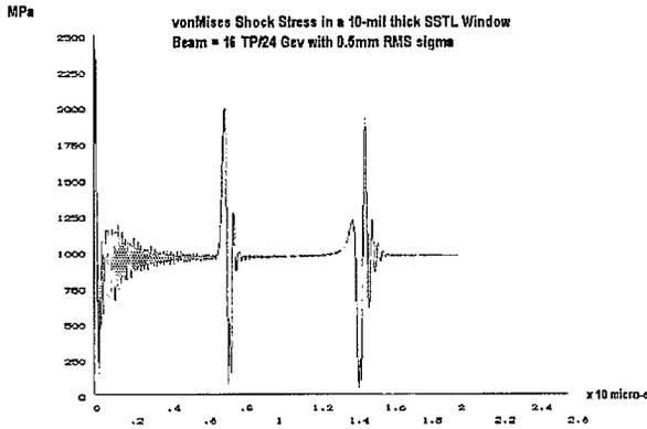
Figure 3: Shock stress in a 10-mil thick Stainless Steel window
