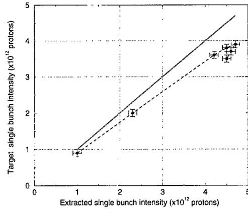
Figure 4: Target beam intensity vs extracted beam intensity. The red line corresponds to a 100 % transmission, to guide the eye.
