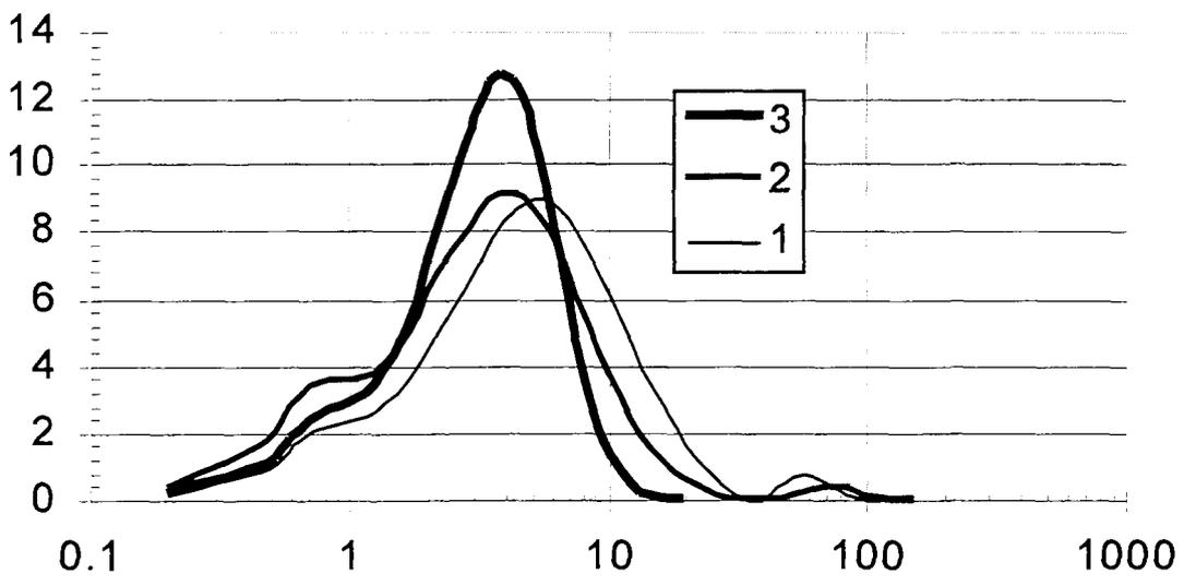
Figure 4. Particle size distribution in bulk samples of air particulate matter, as collected at the Vienna General Hospital (AKH), and after one to three passes through the air-jet mill.
