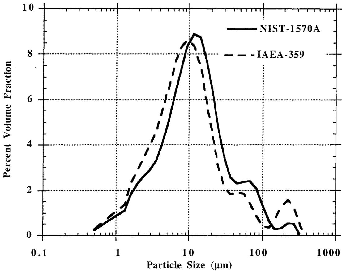
Figure 1. Particle size distribution in IAEA-359, Cabbage, and NIST SRM 1570a, Spinach, after preparation by air-jet milling.
