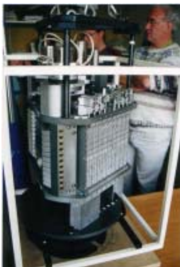
Figure 7. The new 3-face monochromator for the IN8 3-axis spectrometer at ILL.
