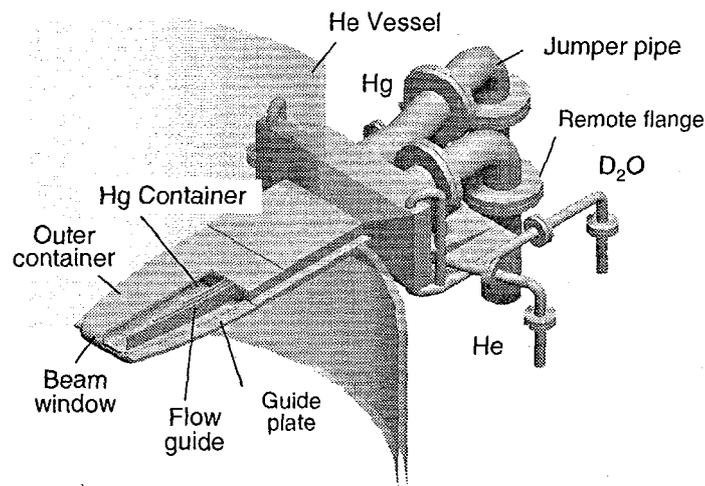
Fig. 2 Target assembly
