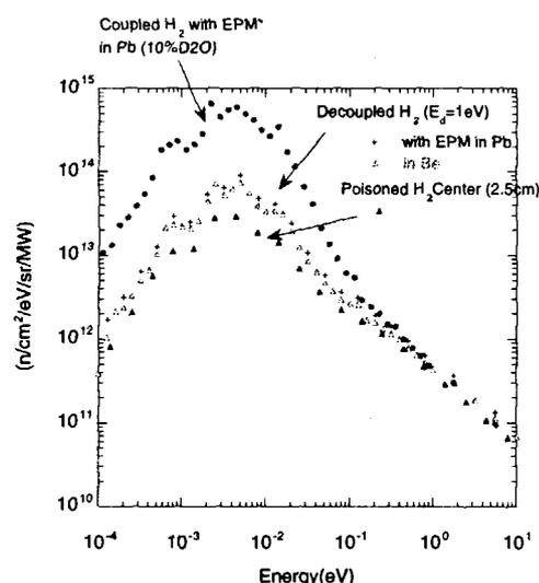
Fig. 6 Typical energy spectra expected to be obtained from the moderator
