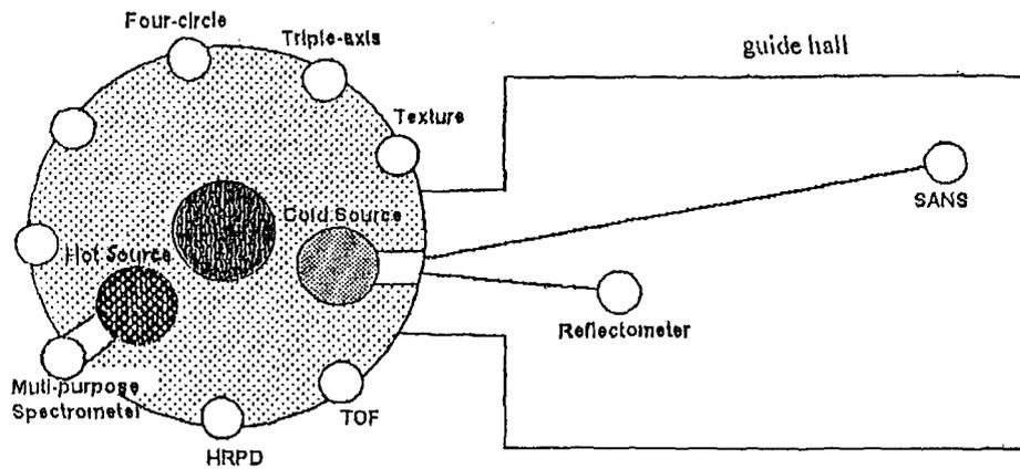
Fig. 2 layout of neutron scattering facilities at CARR
