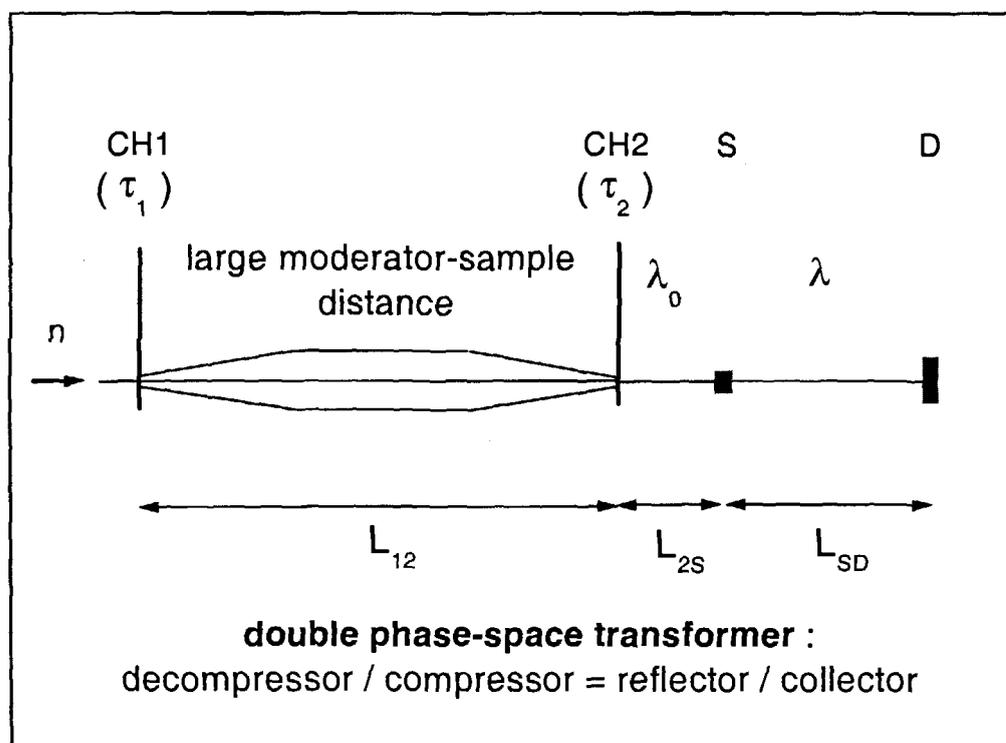
**Fig. 4** Schema of a double phase-space transformer starting with a beam decompressor for the purpose of minimizing transmission losses upon beam transport over a large distance, and ending with a compressor for focussing the beam at the second chopper.
