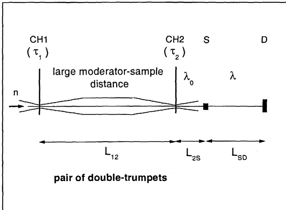
**Fig. 5** Schematic sketch of a pair of double-trumpets implemented at the two principal choppers for intensity-resolution optimization; see discussion in the text.
