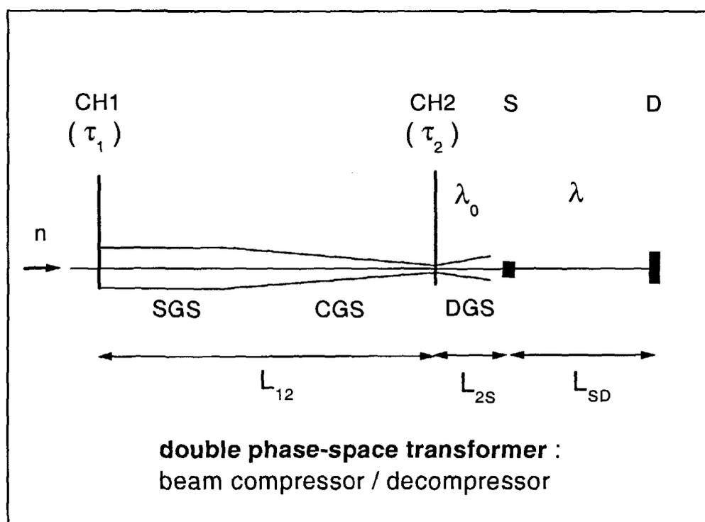
**Fig. 3** Schematic view of a double-trumpet consisting of a pair of converging (CGS) and diverging (DGS) neutron guide sections with the purpose of compressing the pulsed beam in space and time at the chopper disk CH2, and subsequently decompressing it, in order to reduce the divergence of the beam at the sample. SGS = straight (parallel-walled) guide section.
