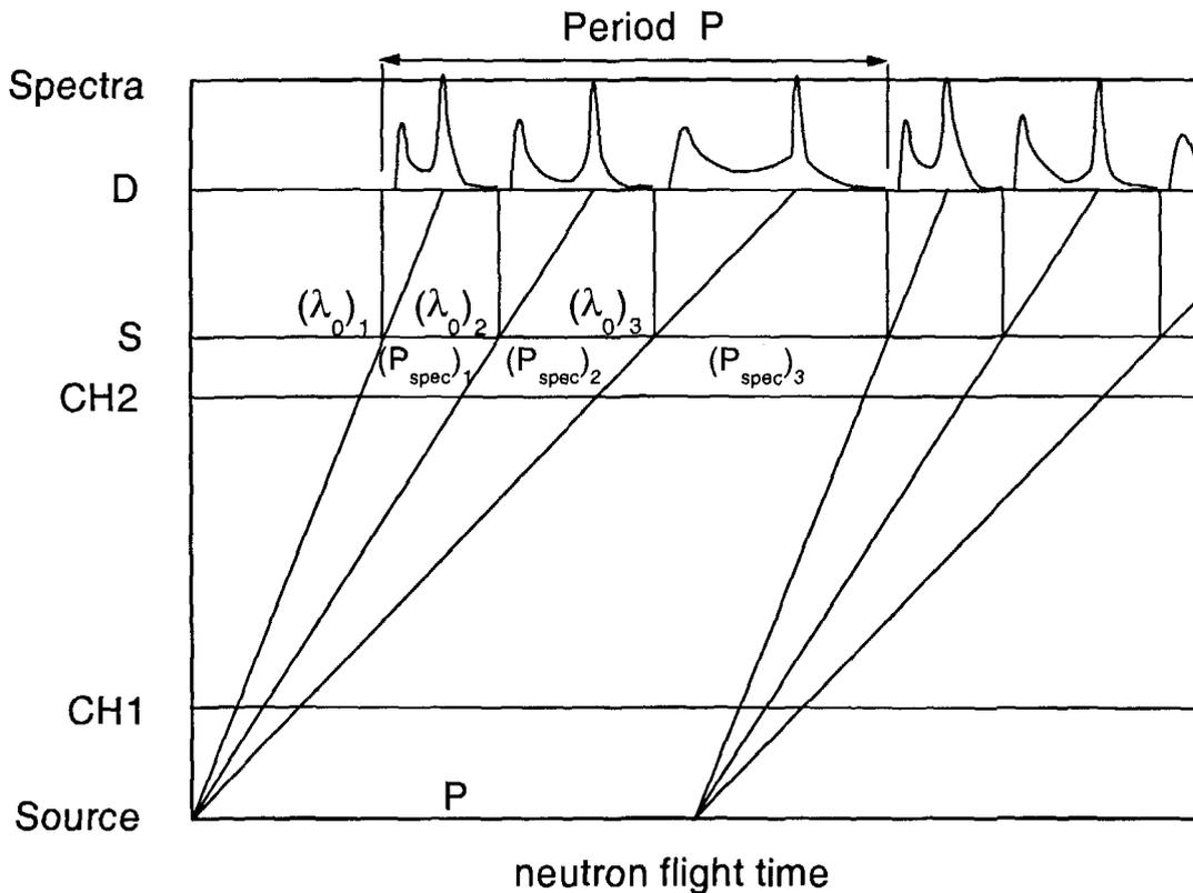
**Fig. 7** Schematic diagram of multichromatic operation of a MTOF spectrometer. Three different incident neutron wavelengths are selected by the chopper cascade so, that the three corresponding spectra of scattered neutrons fill consecutively the period defined by a low pulsed source frequency. The sum of the 3 spectral periods is equal to the source period P.
