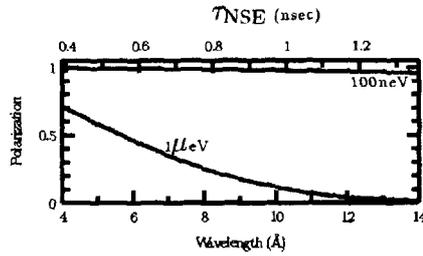
Figure 7: Polarization of NSE signal for MSS-NSE via neutron wavelength.
