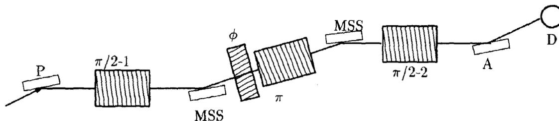
Figure 5: The set up for estimation of thickness and homogeneity of the gap layer.
