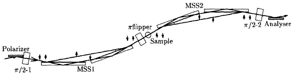
Figure 2: Structure of spin echo spectrometer using MSS.
