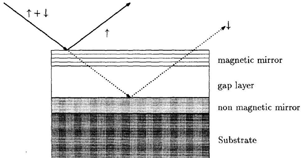
Figure 1: Structure of multilayer spin splitter (MSS).
