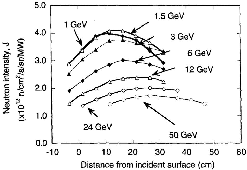
Fig. 7 Time-integrated slow-neutron intensities,  $J$ , for the coupled  $H_2$  mod. with EPM in the Pb reflector as a function of proton energy and position relative to the target (distance from incident surface).
