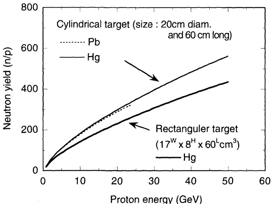
Fig. 5 Comparison of proton energy dependence of leakage neutrons of different target shapes.
