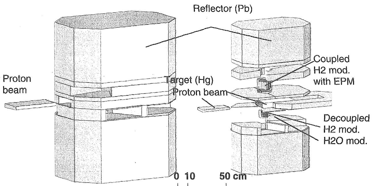
Fig. 3 Calculation model of full system (Target-moderator-reflector).
