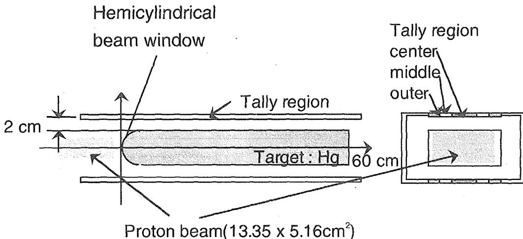
Fig. 2 Calculation model for bare target system.
