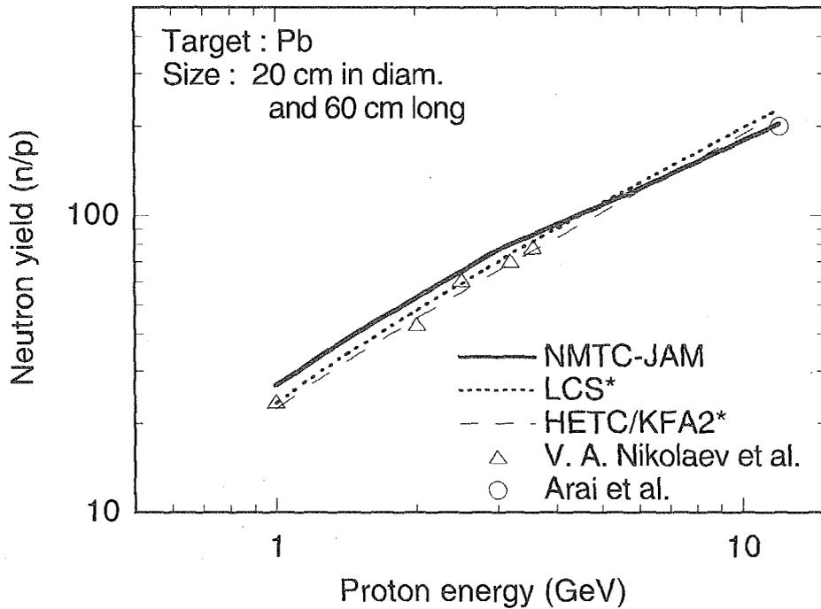
Fig. 1 Comparison of measured and calculated neutron yields.
