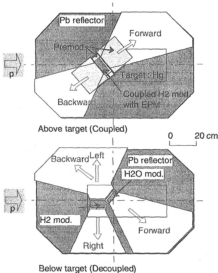
Fig. 4 Calculation model of full system (Target-moderator-reflector).
