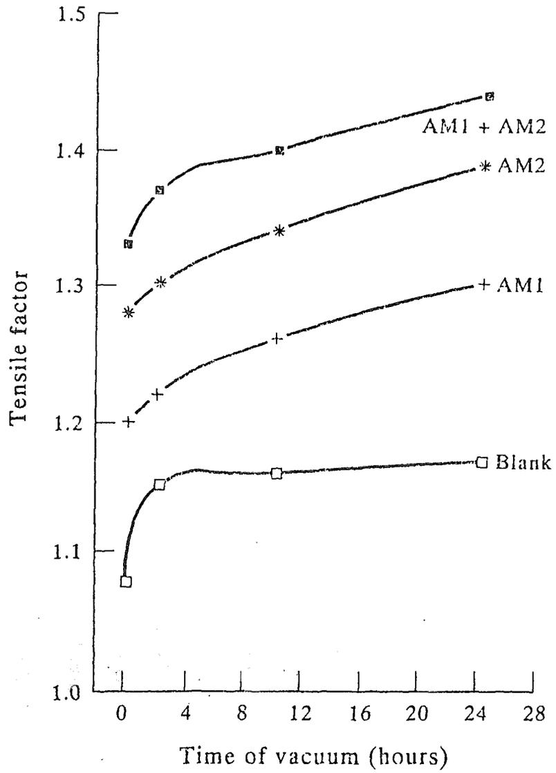
Fig.10 Tensile strength factor of the composites prepared with different impregnating solutions against vacuum time.(TS of simul = 3770 kg/m<sup>2</sup>).
