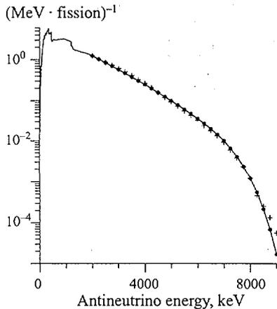
Fig. 1. Reactor antineutrino energy spectrum (contributions to the number of fissions:  $^{235}\text{U}$  — 58%,  $^{239}\text{Pu}$  — 30%,  $^{238}\text{U}$  — 7%,  $^{241}\text{Pu}$  — 5%); curve ( $E < 2$  MeV) — calculation [1, 2]; circles ( $E > 2$  MeV) — measurement [3] at reactor (Rovno); crosses ( $E > 2$  MeV) — standard  $\bar{\nu}_e$  spectrum (from electron spectra [4, 5])
