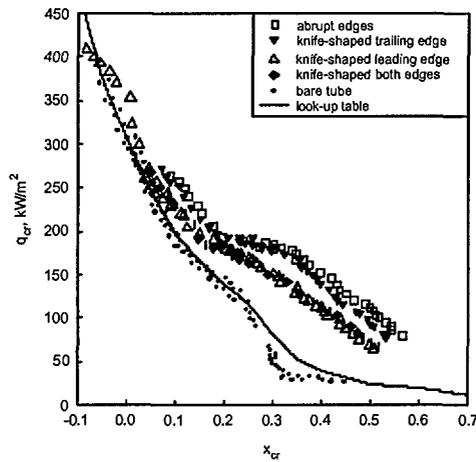
Fig. 3a. Effect of critical quality on CHF in tube with/without flow obstructions: R-134a,  $p=1.67$  MPa,  $G=2000$  kg/m<sup>2</sup>s,  $L=0.45$ -2 m.
