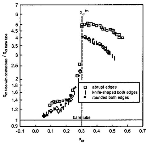
Fig. 7b. Effect of critical quality on CHF enhancement in tube with flow obstructions: R-134a,  $p=1.67$  MPa,  $G=2000$  kg/m<sup>2</sup>s,  $L=0.45$ -2 m.
