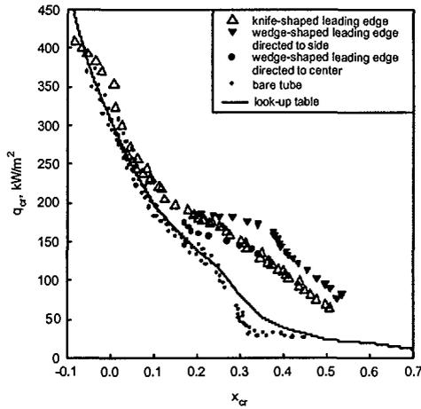
Fig. 5a. Effect of critical quality on CHF in tube with/without flow obstructions: R-134a,  $p=1.67$  MPa,  $G=2000$  kg/m<sup>2</sup>s,  $L=0.45$ -2 m.
