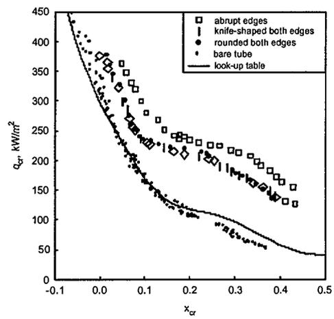
Fig. 8a. Effect of critical quality on CHF in tube with/without flow obstructions: R-134a,  $p=1.67$  MPa,  $G=3000$  kg/m<sup>2</sup>s,  $L=0.45$ -2 m.
