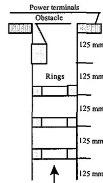
Fig. 1. Test section with flow obstructions.
