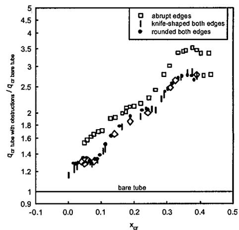
Fig. 8b. Effect of critical quality on CHF enhancement in tube with flow obstructions: R-134a,  $p=1.67$  MPa,  $G=3000$  kg/m<sup>2</sup>s,  $L=0.45$ -2 m.
