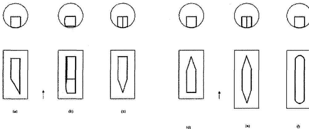
Fig. 2. Flow obstructions – square bars (one side rounded,  $\epsilon=24\%$ ) with various edges: (a) wedge-shaped leading edge directed to side; (b) the same, directed to center; (c) knife-shaped leading edge; (d) knife-shaped trailing edge; (e) knife-shaped both edges; (f) rounded both edges.
