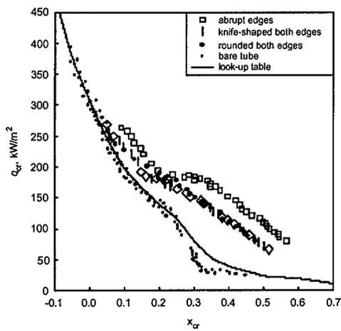
Fig. 7a. Effect of critical quality on CHF in tube with/without flow obstructions: R-134a,  $p=1.67$  MPa,  $G=2000$  kg/m<sup>2</sup>s,  $L=0.45$ -2 m.
