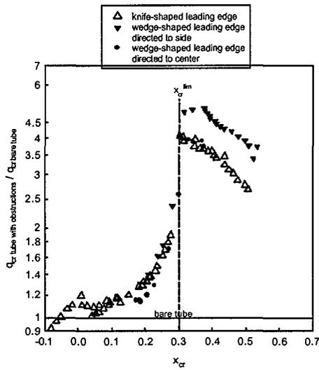
Fig. 5b. Effect of critical quality on CHF enhancement in tube with flow obstructions: R-134a,  $p=1.67$  MPa,  $G=2000$  kg/m<sup>2</sup>s,  $L=0.45$ -2 m.
