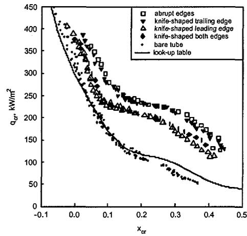
Fig. 4a. Effect of critical quality on CHF in tube with/without flow obstructions: R-134a,  $p=1.67$  MPa,  $G=3000$  kg/m<sup>2</sup>s,  $L=0.45$ -2 m.
