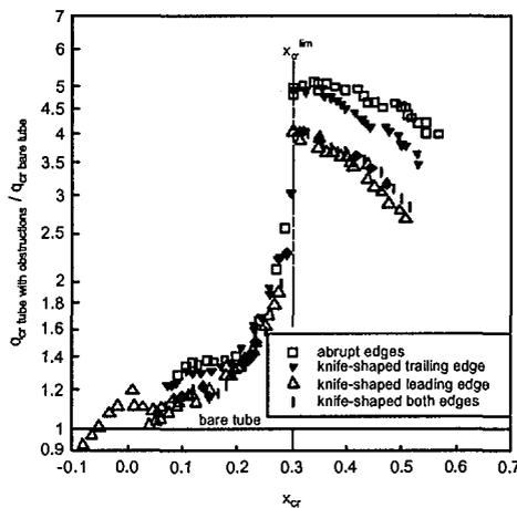
Fig. 3b. Effect of critical quality on CHF enhancement in tube with flow obstructions: R-134a,  $p=1.67$  MPa,  $G=2000$  kg/m<sup>2</sup>s,  $L=0.45$ -2 m.
