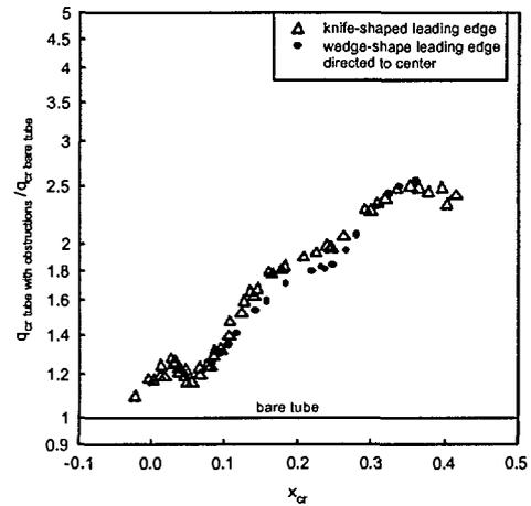
Fig. 6b. Effect of critical quality on CHF enhancement in tube with flow obstructions: R-134a,  $p=1.67$  MPa,  $G=3000$  kg/m<sup>2</sup>s,  $L=0.45$ -2 m.
