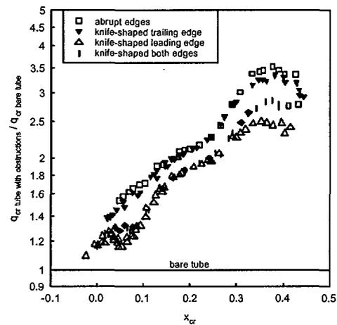
Fig. 4b. Effect of critical quality on CHF enhancement in tube with flow obstructions: R-134a,  $p=1.67$  MPa,  $G=3000$  kg/m<sup>2</sup>s,  $L=0.45$ -2 m.
