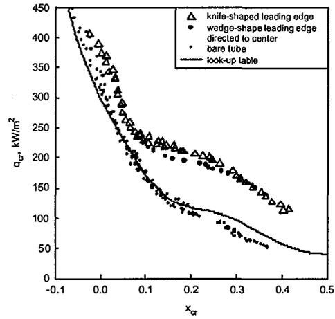
Fig. 6a. Effect of critical quality on CHF in tube with/without flow obstructions: R-134a,  $p=1.67$  MPa,  $G=3000$  kg/m<sup>2</sup>s,  $L=0.45$ -2 m.
