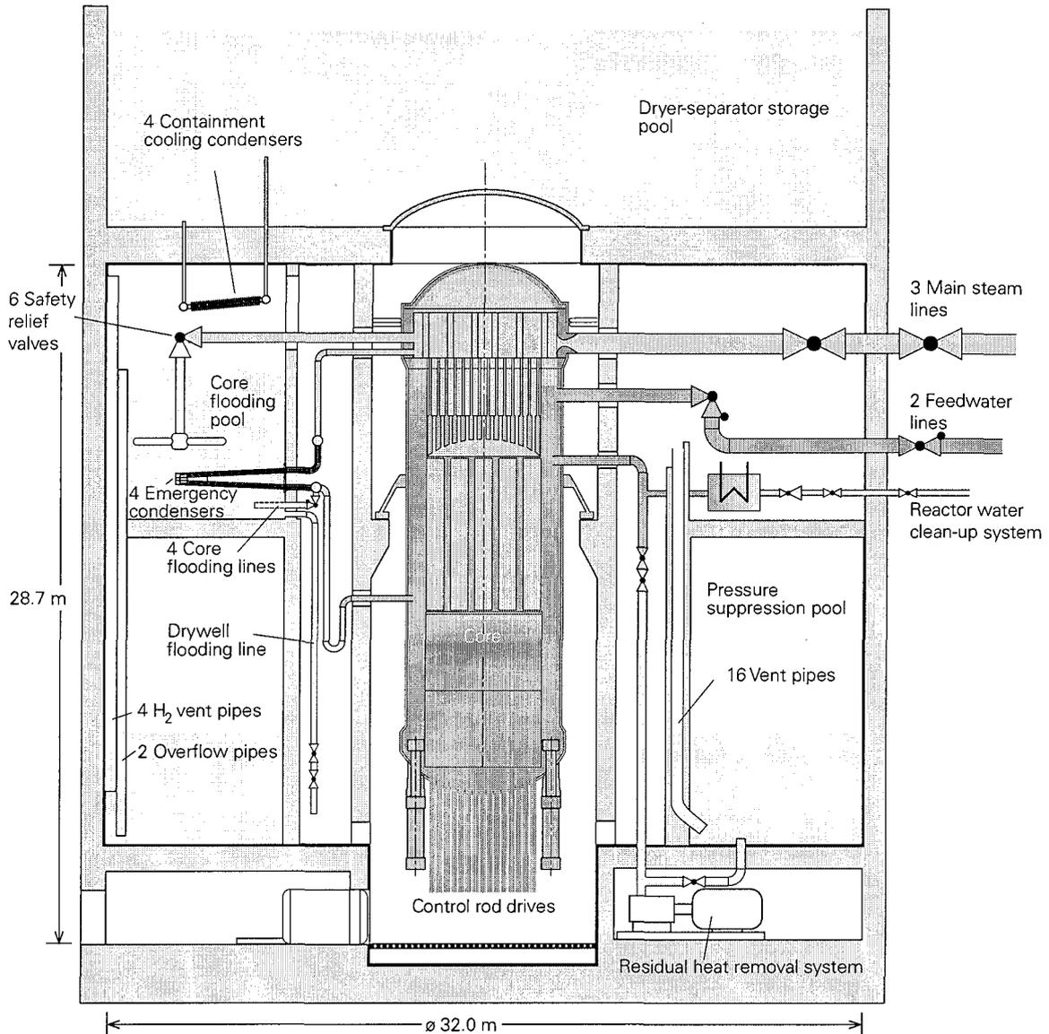
Fig. 2: Containment with active and passive safety systems
