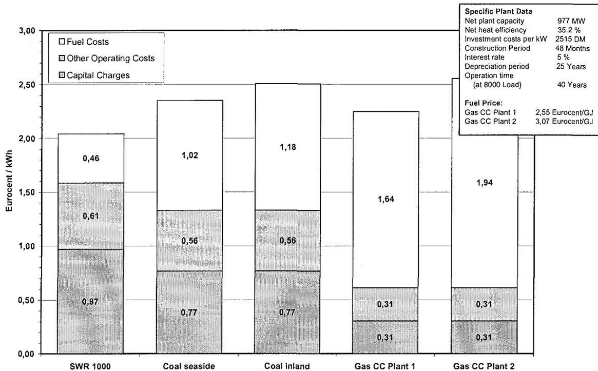
Fig. 5: Comparison of power generating costs
