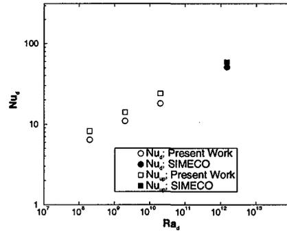
Figure 10: The average Nusselt number as a function of the Rayleigh number  $L_{12} = 8 : 18$ ,  $Q_{v,1} = Q_{v,2}$
