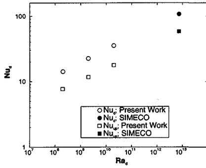
Figure 9: The average Nusselt number as a function of the Rayleigh number.  $L_{12} = 4 : 22$ ,  $Q_{v,1} = Q_{v,2}$
