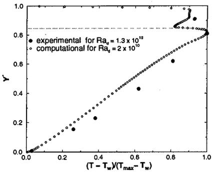
Figure 15: The time average centerline temperature profiles for  $L_{12} = 4 : 22$ . Heat Generation in both layers.
