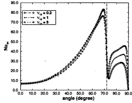
Figure 18: Effect of viscosity ratio on the sidewall Nusselt number distribution for  $\kappa_1 = \kappa_2$ ,  $Q_{v,1} = Q_{v,2}$ .
