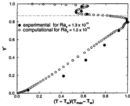
Figure 13: The time average centerline temperature profiles for  $L_{12} = 4 : 26$ . Heat generation in bottom layer.
