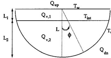
Figure 8: Problem formulation and boundary conditions employed in CFD simulations
