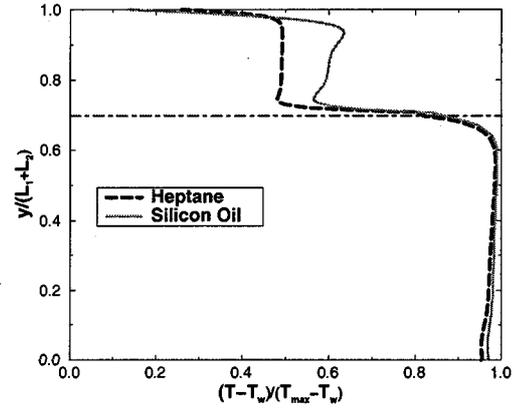
Figure 7: Centerline temperatures for  $L_{12} = 0.433$ ,  $Ra_d = 1.3 \cdot 10^7$
