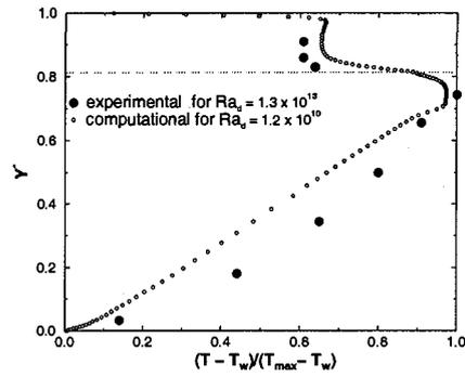
Figure 14: The time average centerline temperature profiles for  $L_{12} = 6 : 26$ . Heat generation in bottom layer.
