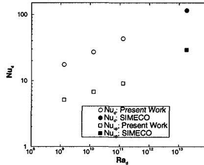
Figure 12: The average Nusselt number as a function of the Rayleigh number for  $L_{12} = 6 : 26$ ,  $Q_{v,1} = 0$
