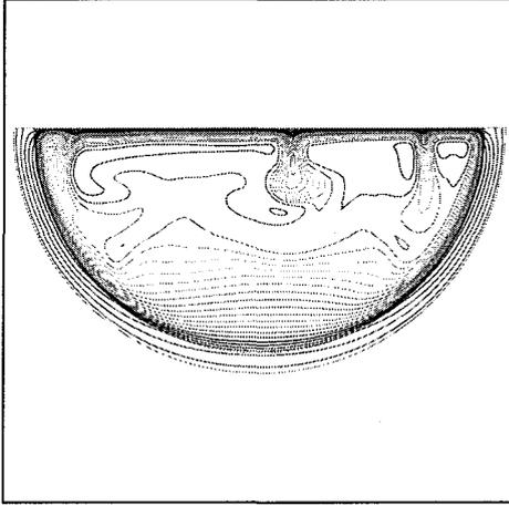
Figure 20: Temperature field for  $Ra = 10^9$ , case 3
