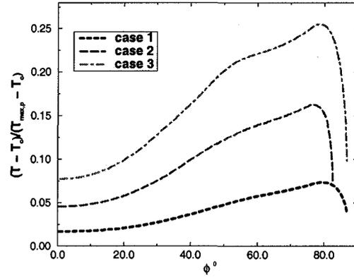
Figure 21: Temperature distribution at the inner surface of the trough
