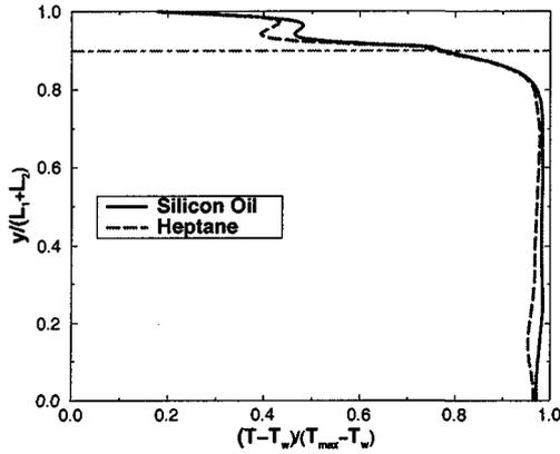
Figure 6: Centerline temperatures for  $L_{12} = 0.11$ ,  $Ra_d = 1.3 \cdot 10^7$
