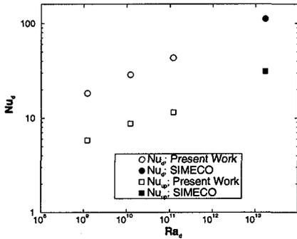
Figure 11: The average Nusselt number as a function of the Rayleigh number.  $L_{12} = 4 : 26$ ,  $Q_{v,1} = 0$
