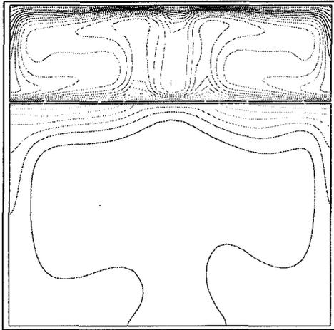
Figure 4: Computed isotherms for Silicon Oil-Water,  $Ra_d = 1.3 \cdot 10^6$ ,  $L_{12} = 0.433$
