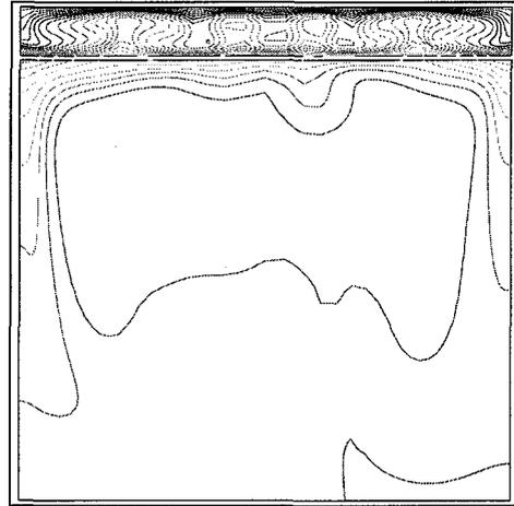
Figure 5: Computed isotherms for Heptane-Water,  $Ra_d = 1.3 \cdot 10^7$ ,  $L_{12} = 0.111$
