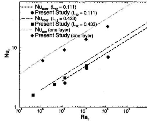
Figure 3: Computed and Experimental Nusselt numbers for Heptane-Water
