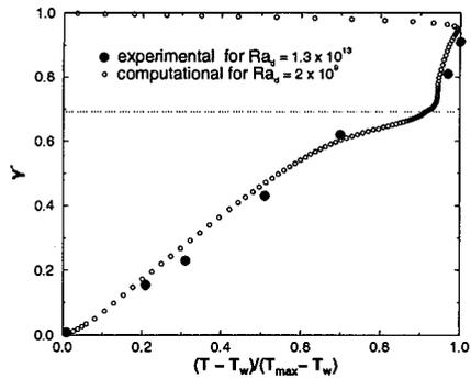
Figure 16: The time average centerline temperature profiles for  $L_{12} = 8 : 18$ . Heat Generation in both layers.
