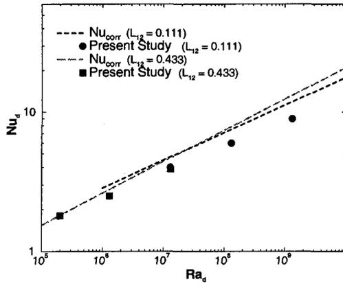
Figure 2: Computed and Experimental Nusselt numbers for Silicon Oil-Water
