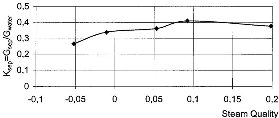
Fig.4. Dependence of Separation Degree in Separation Chamber upon Steam Quality in the Tractive Pipe Inlet at  $G_{min}=9\text{kg/s}$ .
