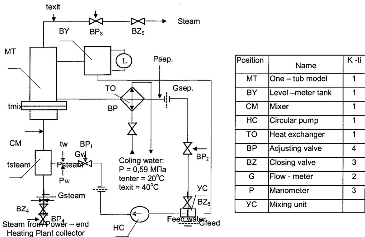
Water from circulating pump NC through the adjusting valve BP1 flows to the mixer CM. Together with water, steam at pressure of  $3.2 + 3.4$  MPa and temperature of  $400 + 420$  °C through closing valve BZ4 (located on the tap of the plant steam collector), flow-meter Gs, and adjustable valve BP4 flows to the mixer, as well.
