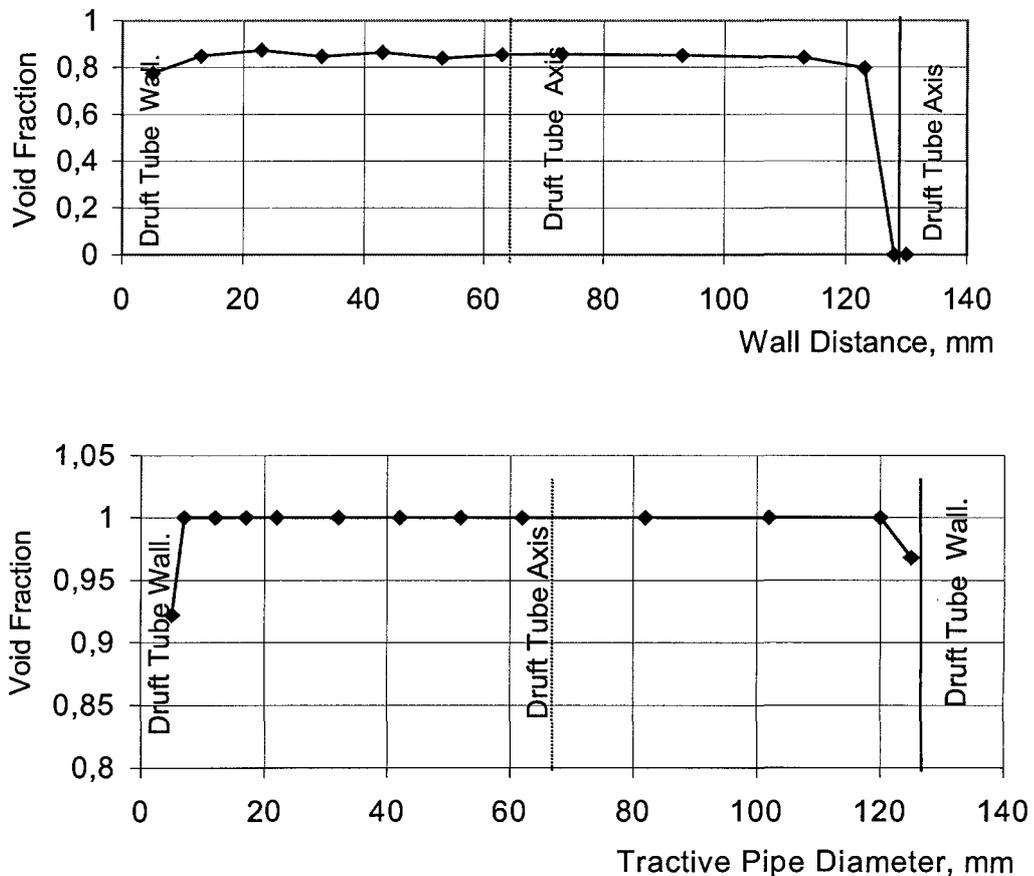
At  $x = 0.12$ , in conditions of steam-water flow equilibrium, the agreement between experimental and predicted data is good. The measured values of mean void fraction in mixing chamber and draught pipe are of 0.53 and 0.88 and calculated – 0.59 and 0.81, correspondingly.
