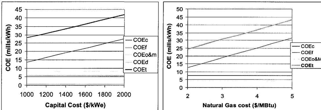
Figure 6: Total, COE<sub>t</sub>, and capital, COE<sub>c</sub>, fuel, COE<sub>f</sub>, and O&M, COE<sub>O&M</sub>, contributions for NP as a function of capital cost and for CCGT as a function of Natural Gas price.
