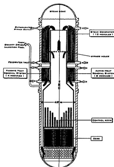
Figure 1: Layout of the NILUS reactor
