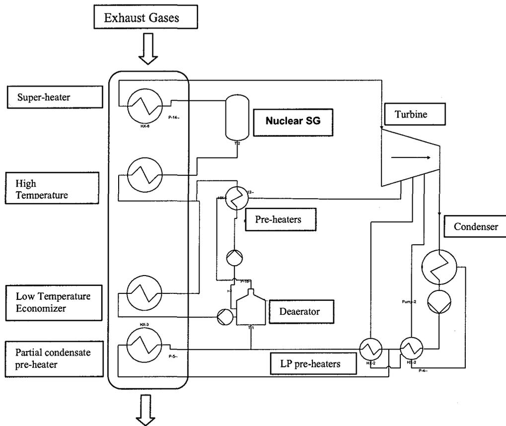
Figure 3: Conceptual scheme of the CNGT
