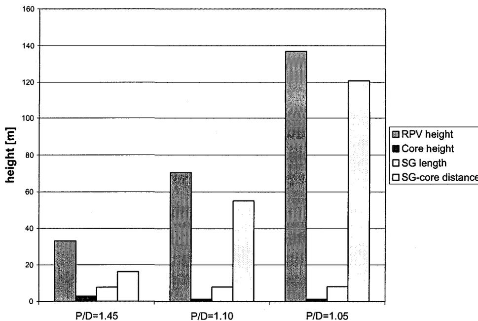
Figure 2: Reactor Pressure Vessel dimensions for IRIS-300MWt core for different P/D ratios.
