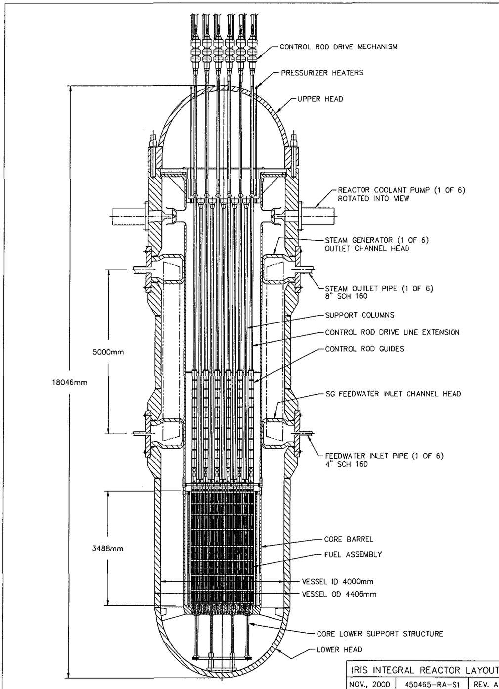
Figure 4: IRIS reactor reference layout
