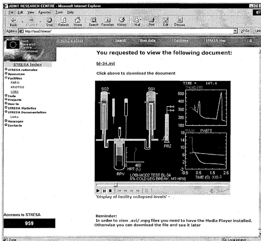
Fig. 7 – Display of measured collapsed levels in the LOBI facility during Test BL-34. It is possible to identify the time of loop seal clearing which determines a temporary core rewetting.
