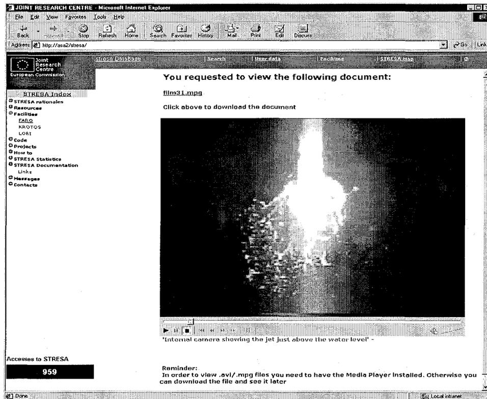
Fig. 8 – A film performed during a FARO test which shows the initial portion of a molten  $\text{UO}_2$  jet at about 3000 K just before entering the water pool
