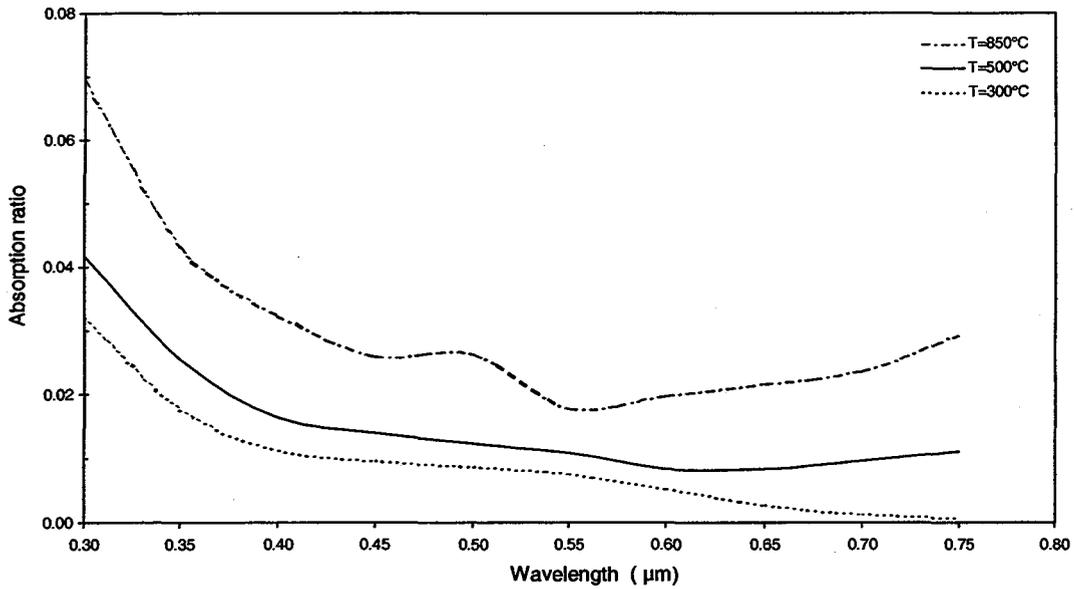
**Fig. 12 : Absorption ratio vs. wavelength;  $2\pi r/\lambda=0.5$**
