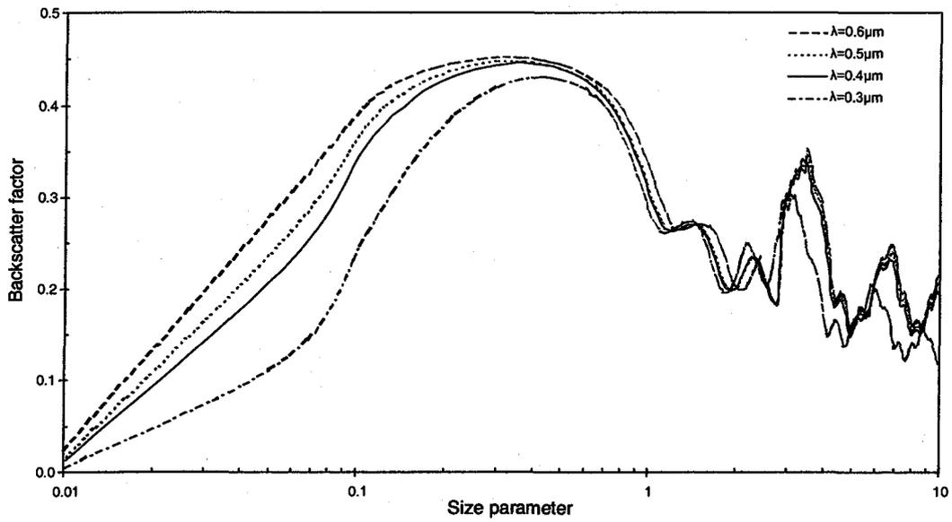
**Fig. 5 : Backscatter factor vs. size parameter;  $T=500^{\circ}\text{C}$**
