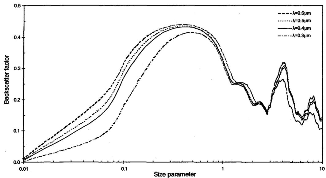
**Fig. 3 : Backscatter factor vs. size parameter; T=850°C**
