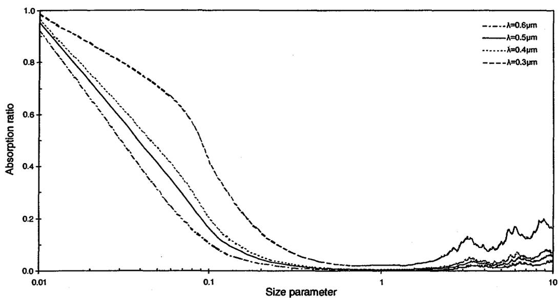
**Fig. 8 : Absorption ratio vs. size parameter; T=300°C**
