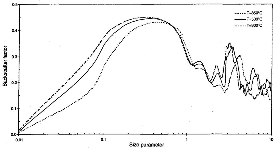
**Fig. 9 : Backscatter factor vs. size parameter;  $\lambda=0.4\mu\text{m}$**
