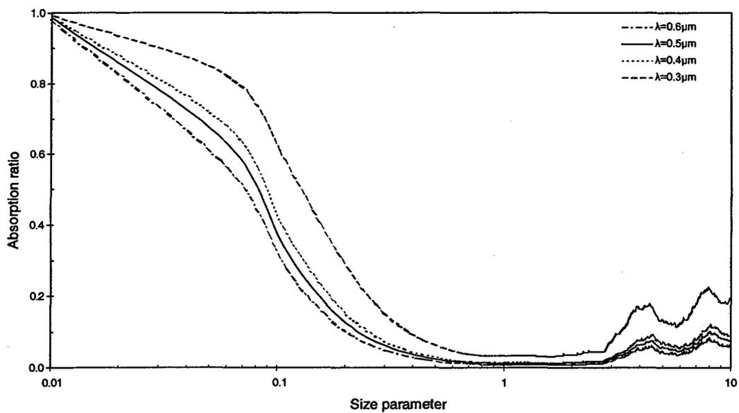
**Fig. 4 : Absorption ratio vs. size parameter; T=850°C**
