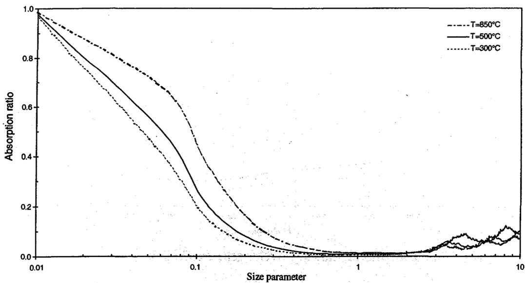
**Fig. 10 : Absorption ratio vs. size parameter;  $\lambda=0.4\mu\text{m}$**
