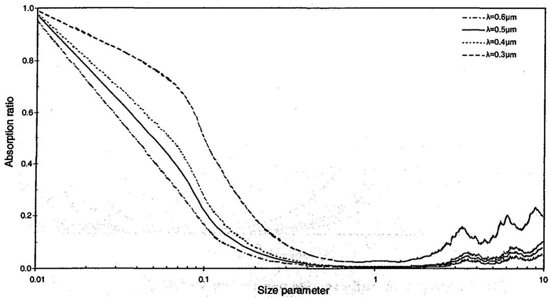
**Fig. 6 : Absorption ratio vs. size parameter;  $T=500^{\circ}\text{C}$**
