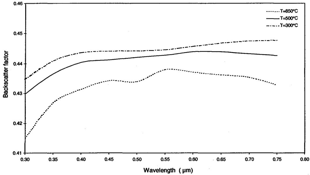
**Fig. 11 : Backscatter factor vs. wavelength;  $2\pi r/\lambda=0.5$**
