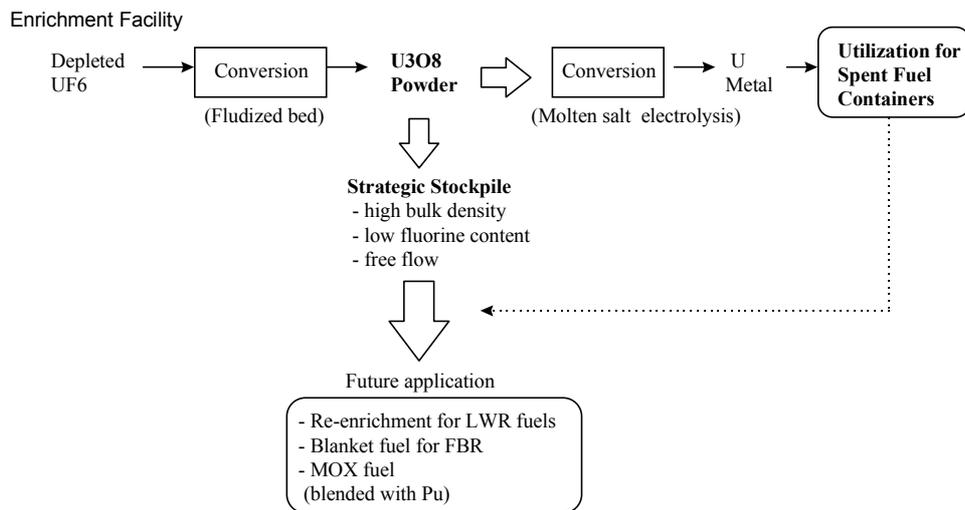
**FIGURE 6.** Option for Depleted uranium recycling
