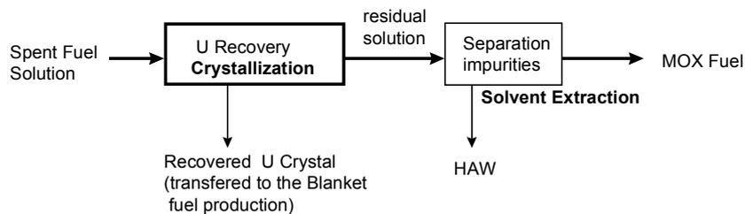
FIGURE 4. A Block Flow of Crystallization Process (Application C)
