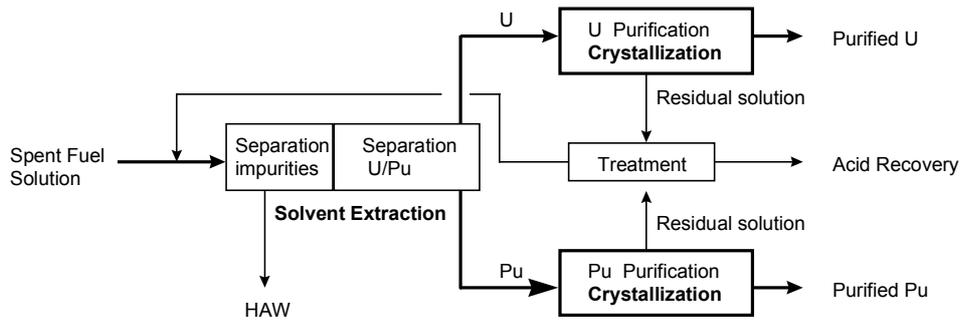
FIGURE 2. A Block Flow of Crystallization Process (Application A)
