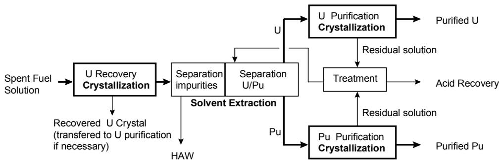
FIGURE 3. A Block Flow of Crystallization Process (Application B)
