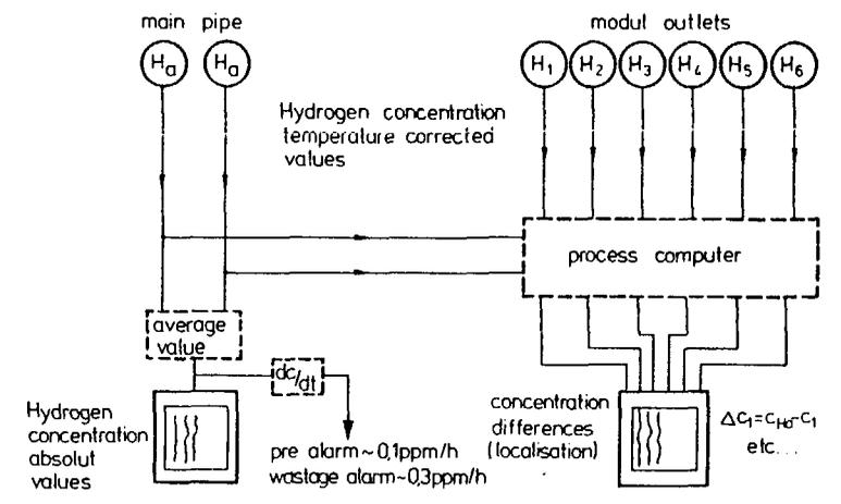
fig.1.5 SNR300 signal processing, Hydrogen detectors
