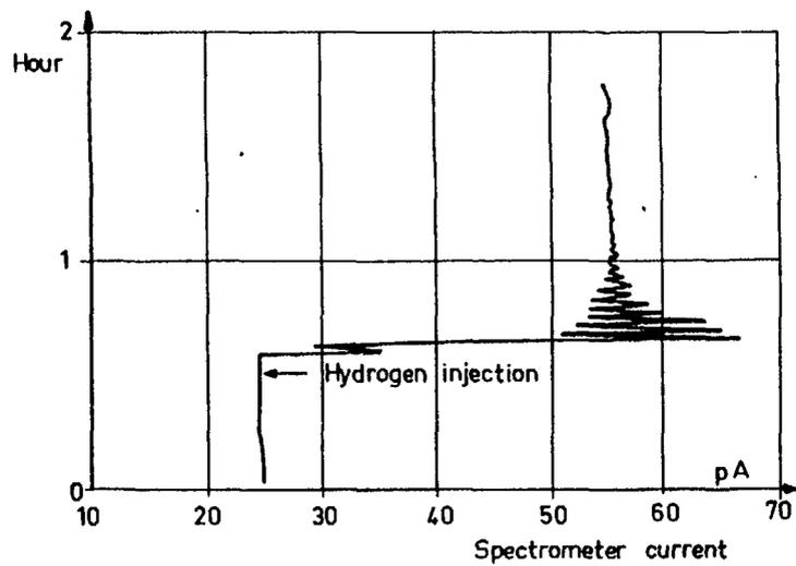
FIG. 6: SUPER PHENIX PROTOTYPE SYSTEM FOR HYDROGEN MEASUREMENT IN SODIUM SPECTROMETER CURRENT AS A FUNCTION OF TIME DURING A HYDROGEN INJECTION.
