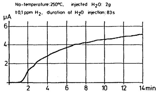
water injection tests at different temperatures (membrane 0,5mm, 54,3cm<sup>2</sup>)
