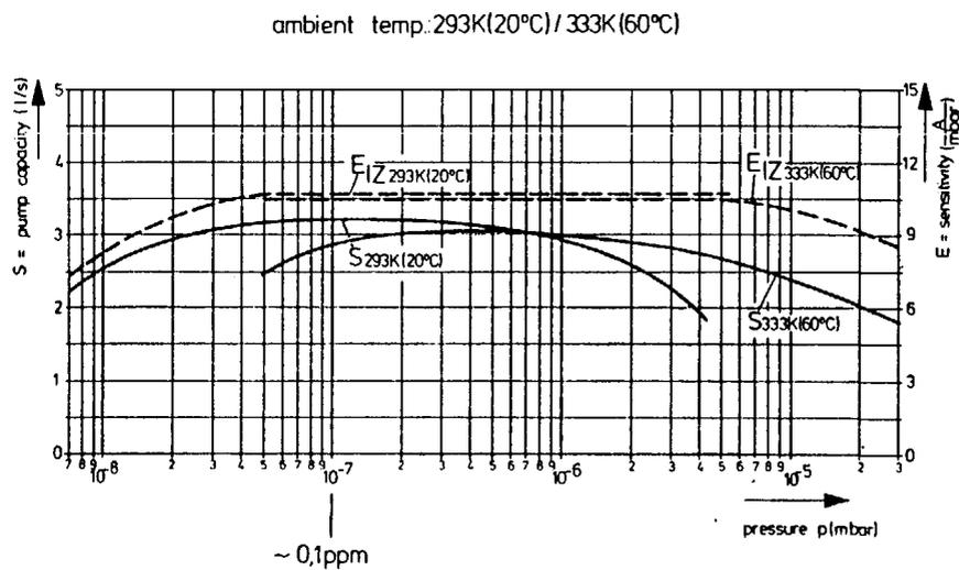
fig.26 pump capacity and sensitivity, ion getter pump IZ2
