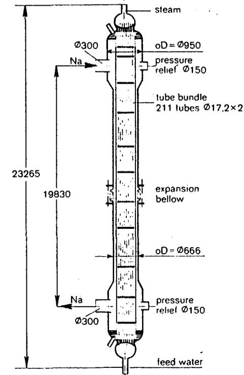
SNR-STRAIGHT TUBE STEAM GENERATOR - EVAPORATOR-
