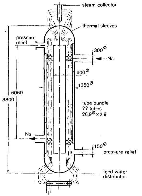
SNR HELICAL COIL STEAM GENERATOR-EVAPORATOR-
