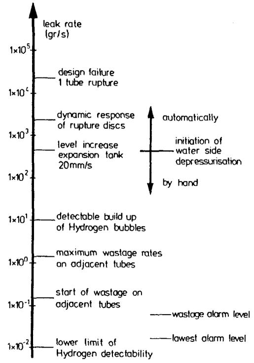
leak detection systems SNR 300
