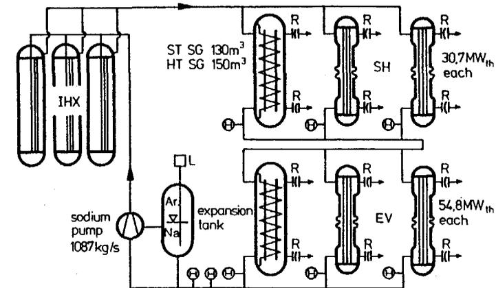
fig.11 secondary heat transfer system
