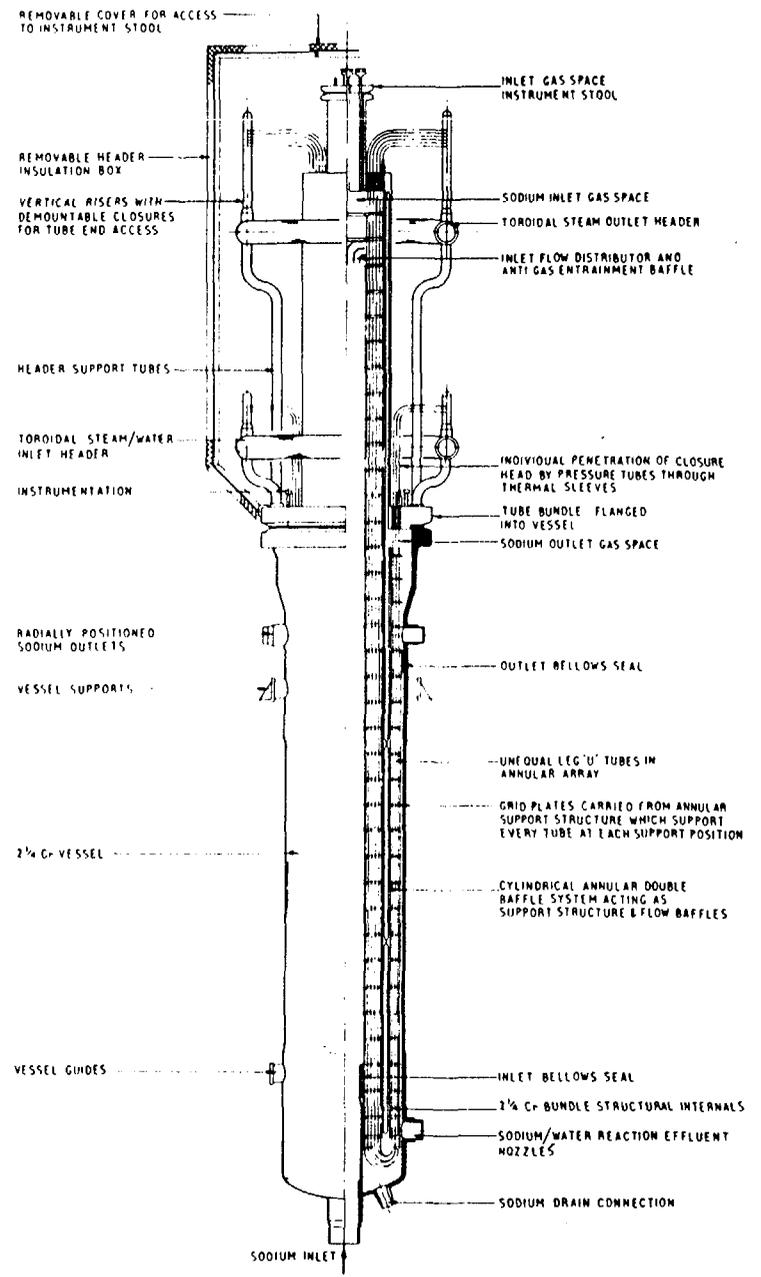
PRINCIPLE FEATURES OF CFR STEAM GENERATOR
