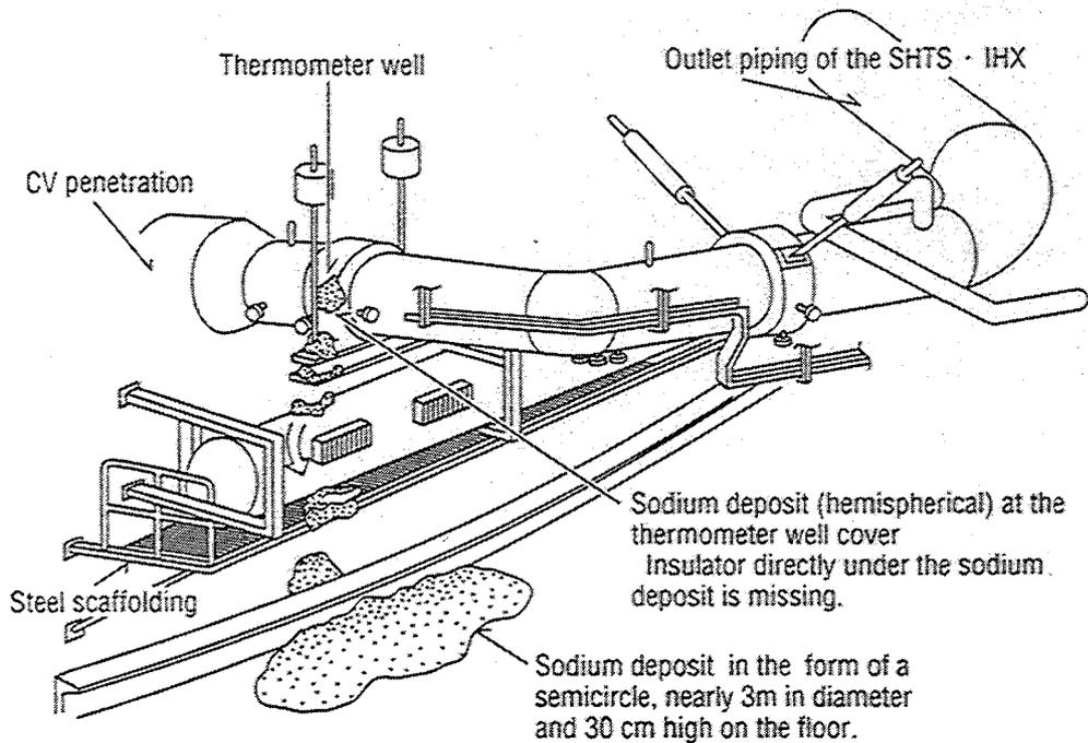
**Fig 3.3 Schematic view of a sodium leak in SHTS C loop piping room**
