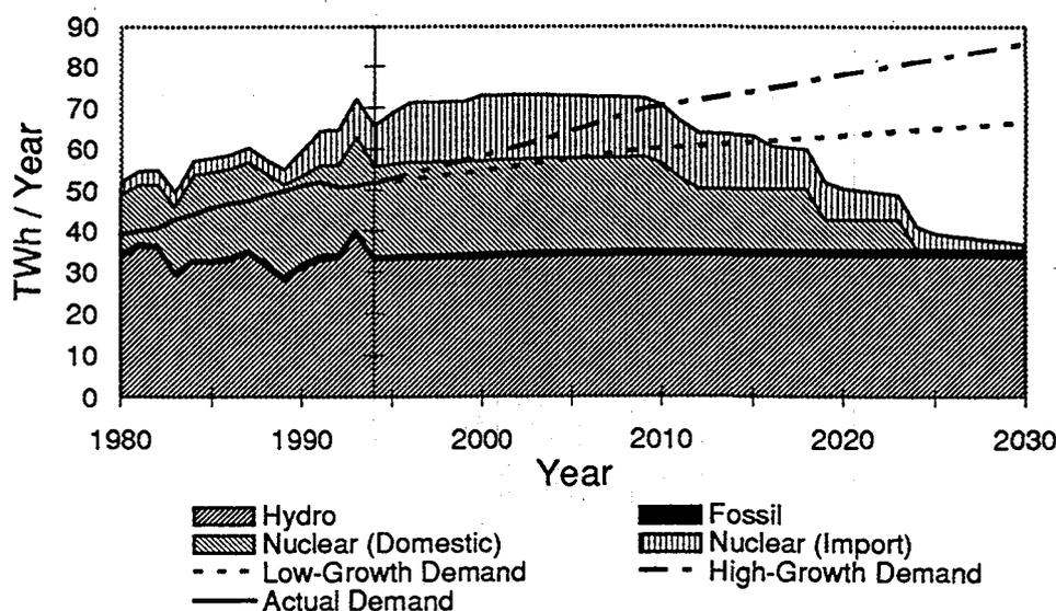
Fig. 1: Electric energy demand cases considered by VSE and the secured yearly electricity supply for the period 1995-2030.
