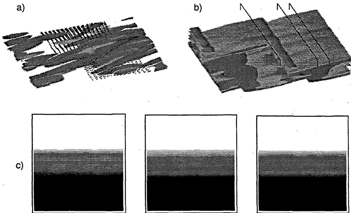
**Fig. 7:** Stably-stratified mixing layer calculation with combined deterministic and random initial conditions for liquid sodium simulation at Richardson number  $Ri = 0.05$ . Vorticity isosurfaces (see a), passive scalar isosurfaces (i.e. surfaces with equal marker substance concentration; see b), and cross-sectional cuts of the passive scalar (see c), at different streamwise locations (as marked in b) are given.
