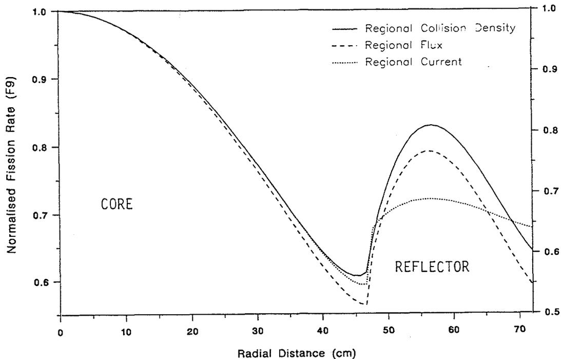
**Fig. 4:** ZONA2-A3 axially centered Pu239 fission rate radial profiles using different homogenisation procedures in the cell calculation
