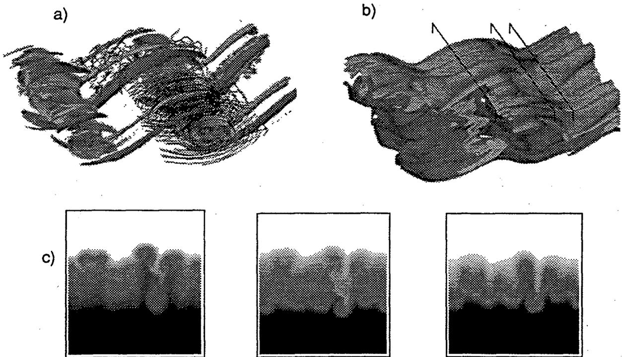
**Fig. 5:** Unstratified mixing layer calculation with combined deterministic and random initial conditions for air simulation at Richardson number  $Ri = 0.00$ . Vorticity isosurfaces (see a), passive scalar isosurfaces (i.e. surfaces with equal marker substance concentration; see b), and cross-sectional cuts of the passive scalar (see c), at different streamwise locations (as marked in b) are given.
