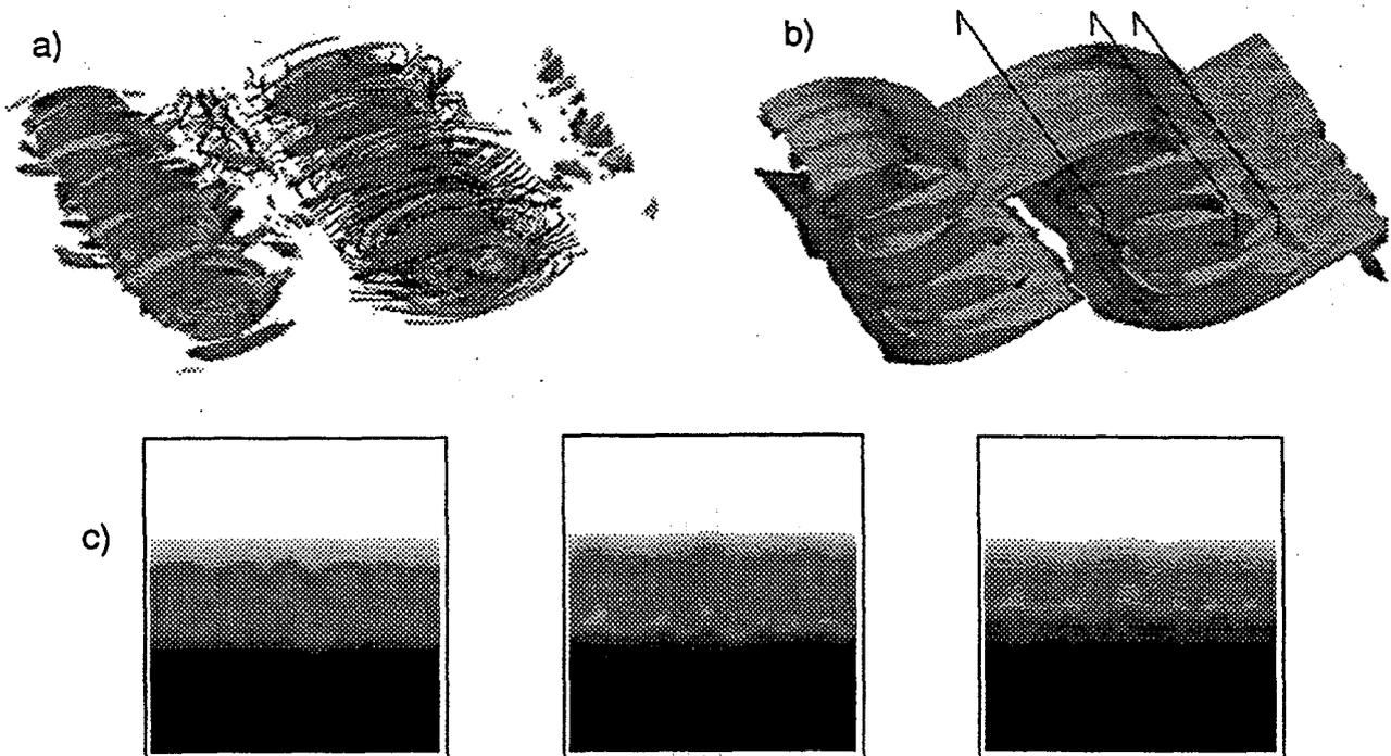
**Fig. 6:** Stably-stratified mixing layer calculation with combined deterministic and random initial conditions for air simulation at Richardson number  $Ri = 0.05$ . Vorticity isosurfaces (see a), passive scalar isosurfaces (i.e. surfaces with equal marker substance concentration; see b), and cross-sectional cuts of the passive scalar (see c), at different streamwise locations (as marked in b) are given.
