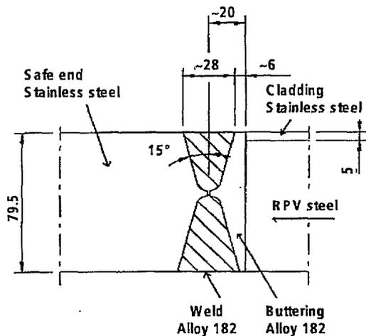
Figure 1. Schematic showing the nozzle to safe end weld. All dimensions are in mm.
